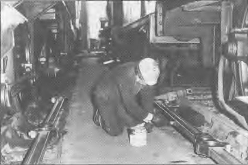
The side rods of the J27 being painted by Dave Whitfield inside Deviation shed on 16 th January (John Hunt)
