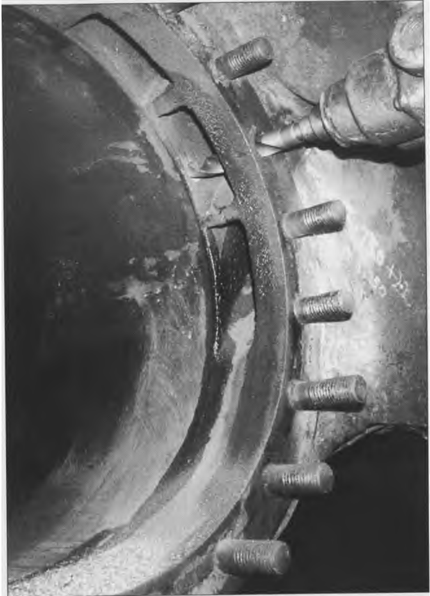
Drilling through the middle cylinder stud hole into the main cylinder block on 5 th January 2001 for an extended stay stud to be fitted, hopefully to restrain any further cracking of the cylinder block (Maurice Johnson)
