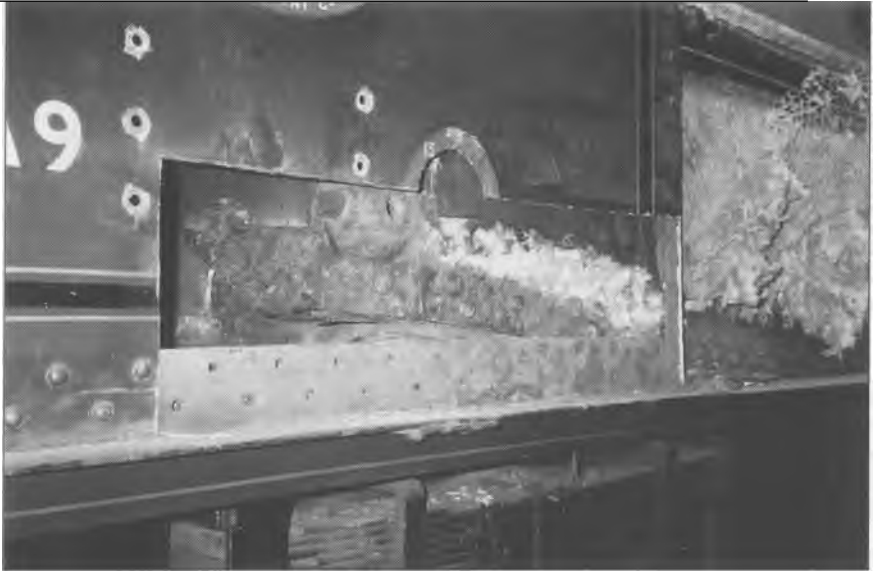
A 44" x 12 " section of 60532 's cab cut away to facilitate rivet replacement in the back right corner of the foundation ring on 12 th January 2001 (Maurice Johnson)
