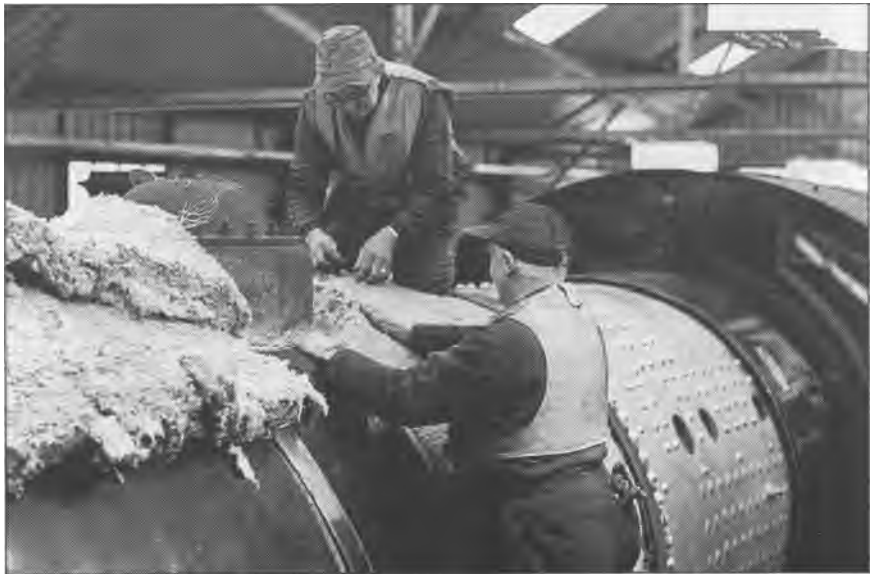
Martin Lloyd and Toni Young fit boiler lagging to the K1 at Grosmont on 3 rd May (Colin Smith)
