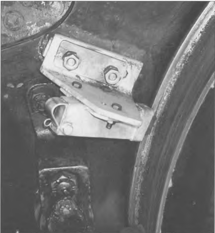
One of the flange lubricators now fitted to the rear driving wheels of the K1 (Maurice Johnson)
