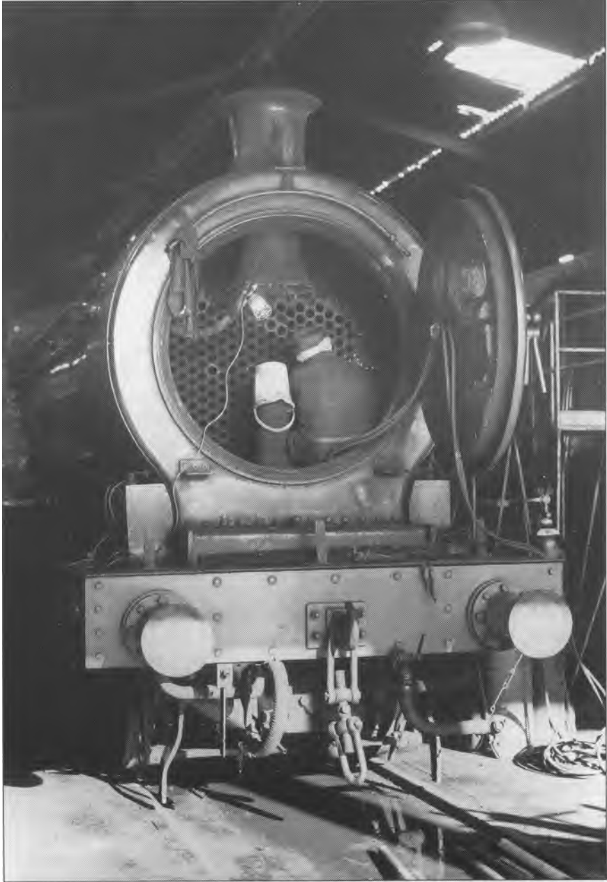
Maurice Johnson working inside the smokebox of the J27 at Grosmont on 28.10.01 preparing the front tubeplate retubing (John Hunt)
