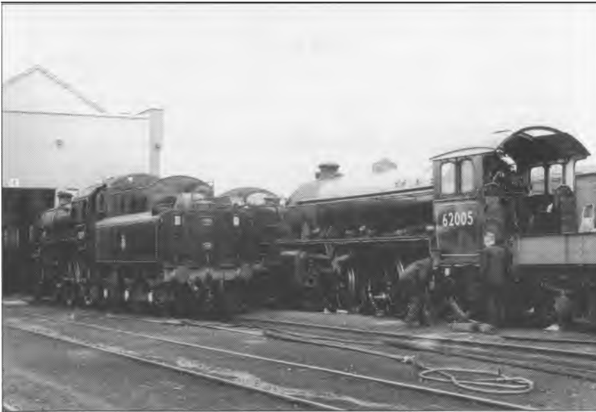
Ian Riley's staff refitting the springs to the K1 at Bury on 13 th June assisted, out of sight, by Fred and Malcolm (John Hunt)
