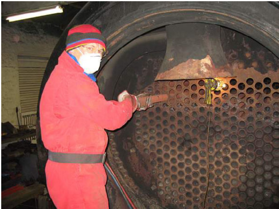
Bernie Lythe posing while pulling tubes out of the J27's boiler on 5 th November (Richard Pearson)
