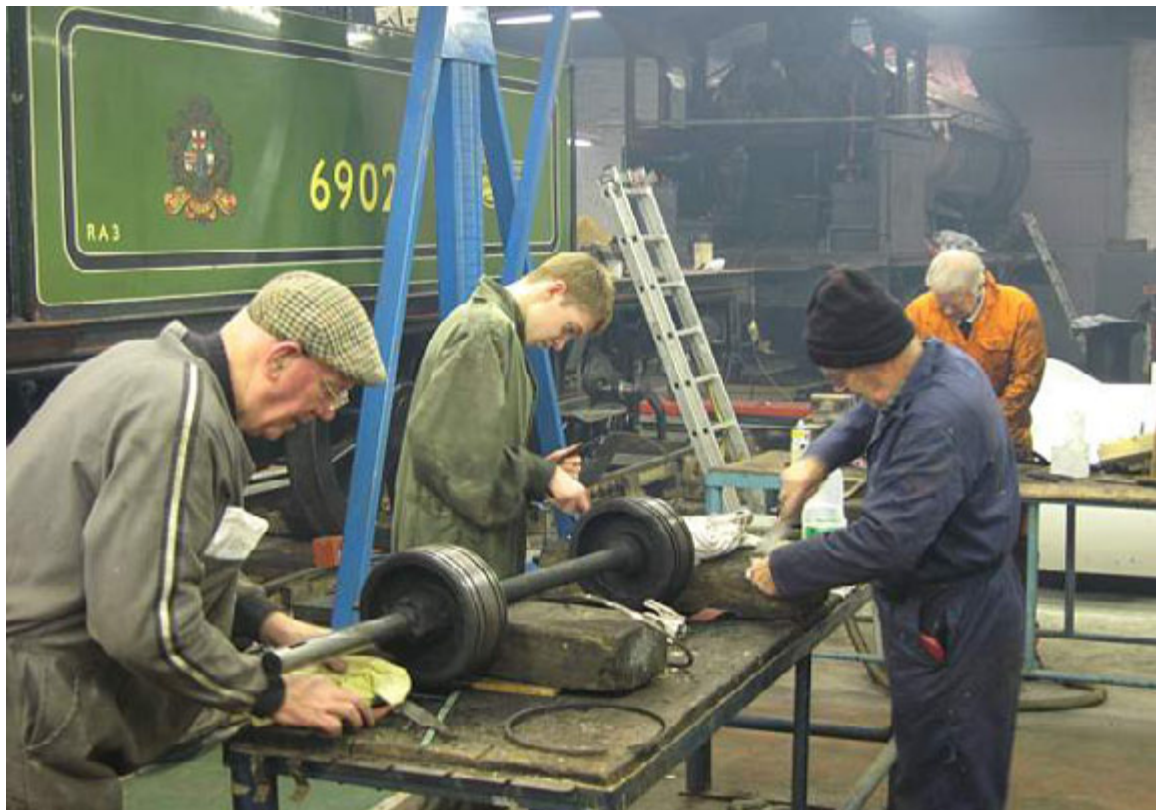
L to R, Nev Barlow, Jason Brown and Brian Swallow working on one of the K1's piston valves at Hopetown; they are busy cleaning the valve heads and the rings. In the background Allan Wilson is repairing the K1's blast pipe spark arrestor screens (Richard Pearson)
