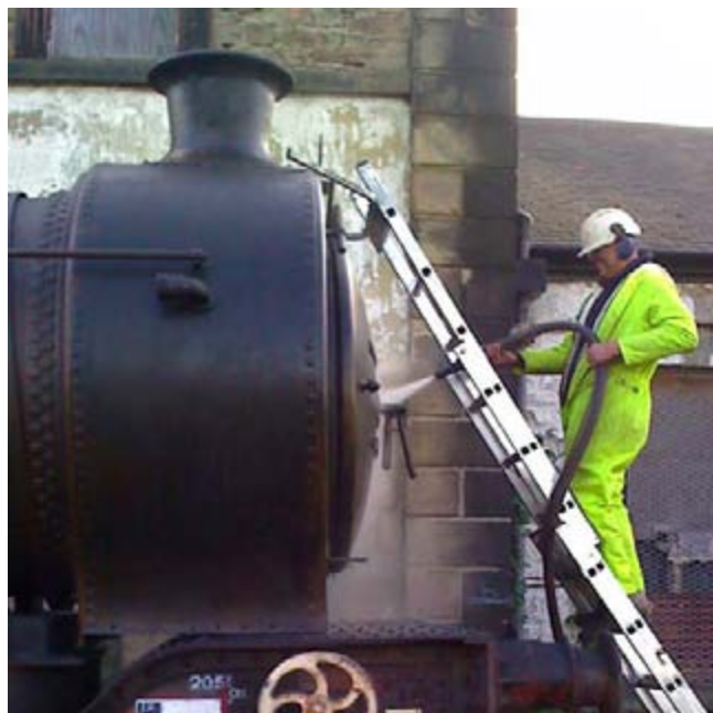
The smokebox being shot blasted on 3 rd October (Nigel Hall)
