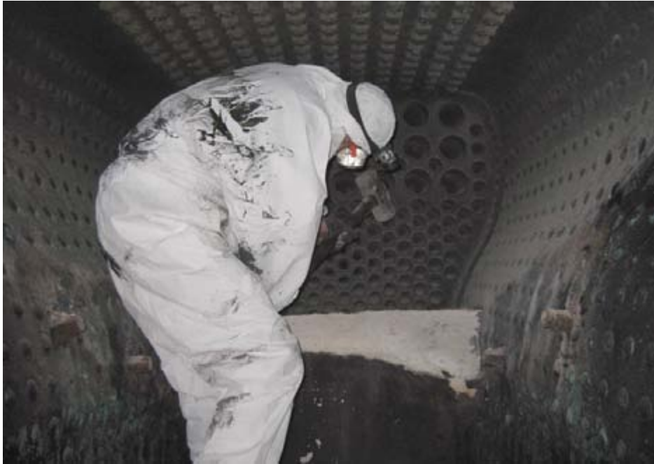
Guy Atkins, suitably attired, removing the concrete arch inside the K1's firebox on 4 th October (Richard Pearson)
