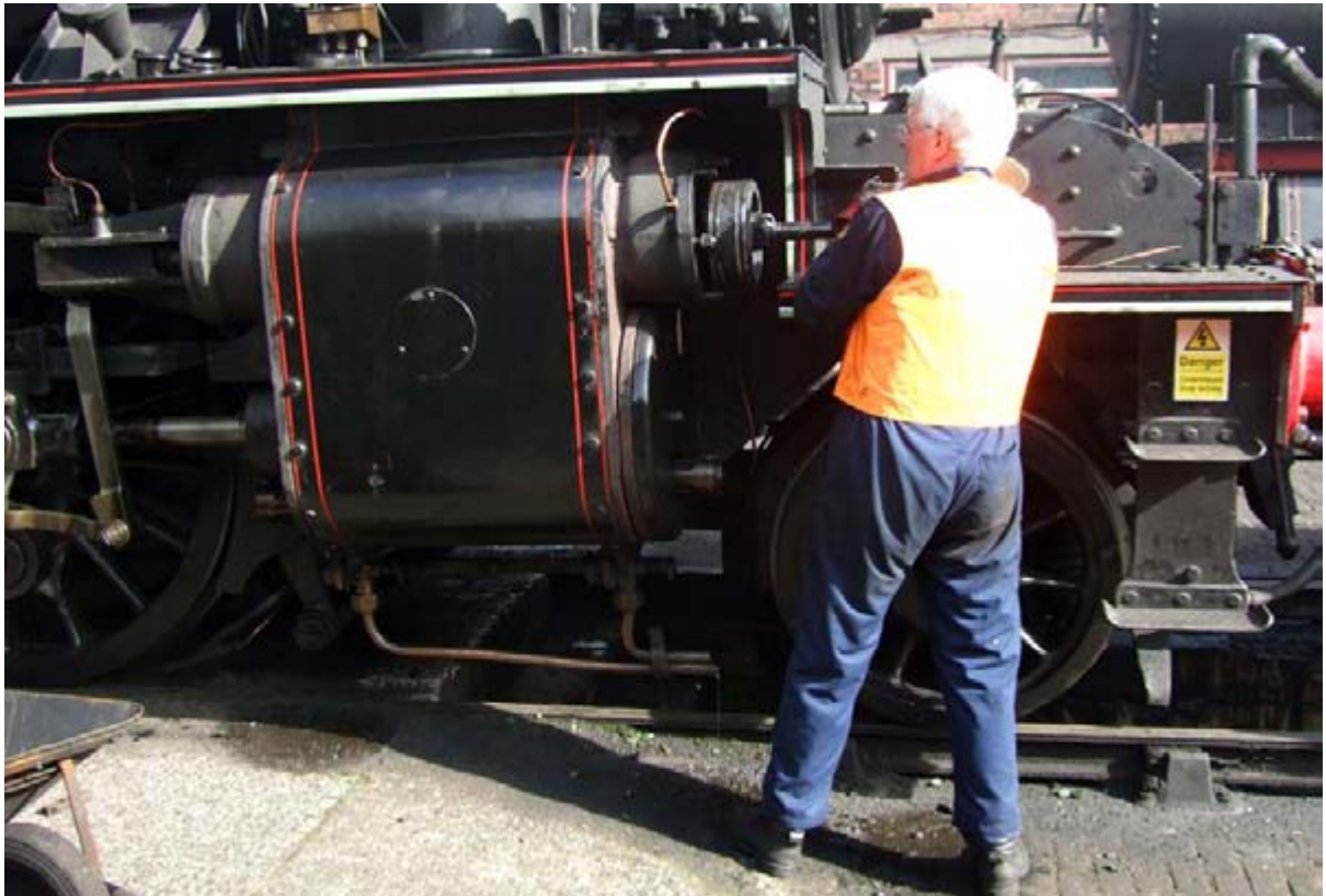
Dave Donegan starts to extract a valve from the K1 on 24 th September (Colin Smith)
