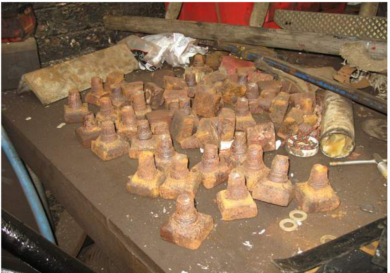
The old roof stay bolts, which are very badly corroded (Richard Pearson)
