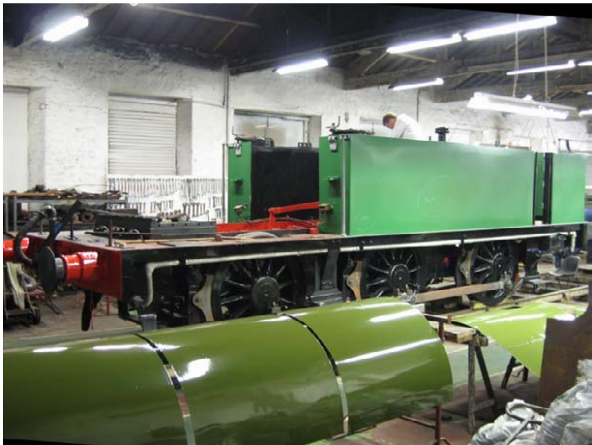
Going green! The boiler cladding sheets in gloss on 13 th October (Richard Pearson)
