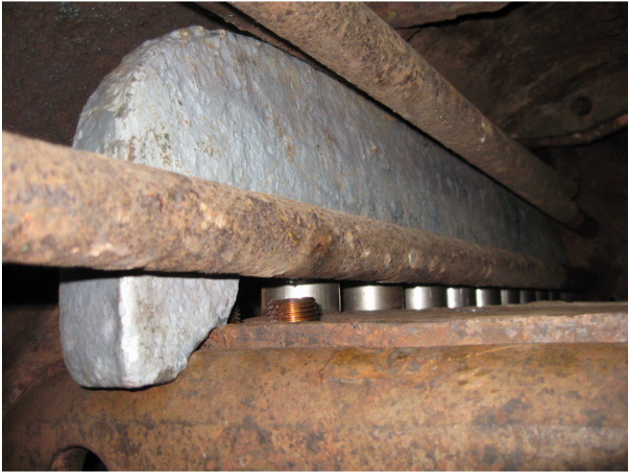
This shot taken from inside the boiler barrel looking across the top of the inner firebox shows the first girder stay back in position. The girder is grey and the new shining ferrule can be seen; the new roof stay bolts screw up from inside the firebox through the ferrule and into the girder to hold it in position (Richard Pearson)
