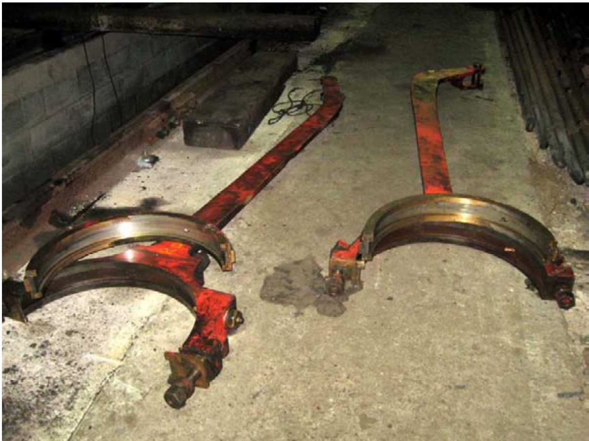
The two Q6 eccentric rods, showing the two halves of the eccentric straps on 9 th March (John Hunt)
