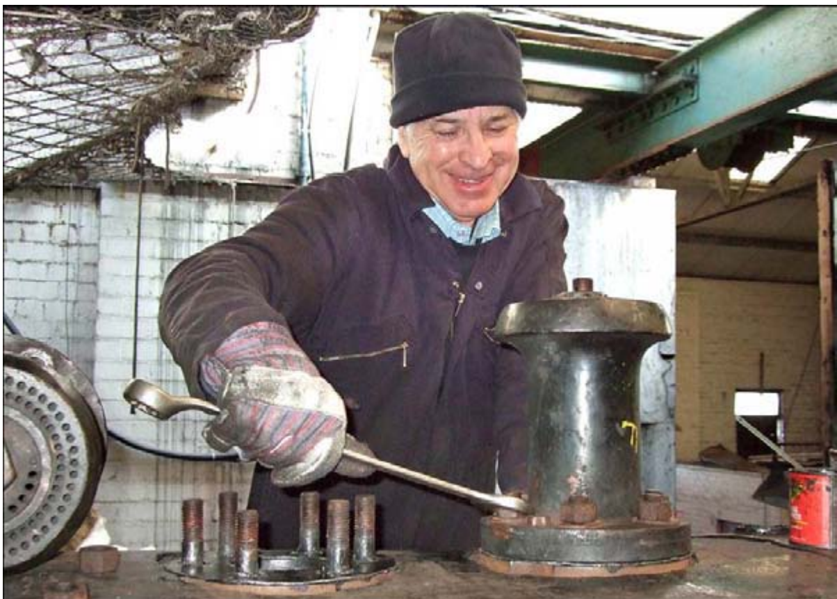
Steve Hyman refits the front safety valve on the K1 at Carnforth on 10 th March (Colin Smith)
