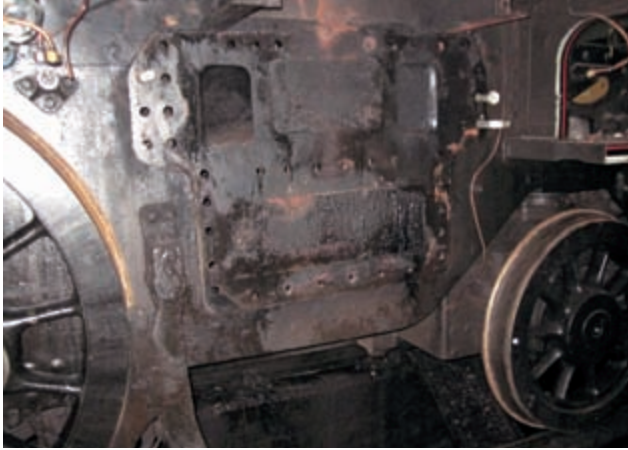
The K1's right hand cylinder removed and showing the two exhaust ports (John Hunt)
