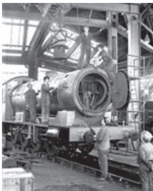
One of the Thornaby working parties refits the chimney (John Boyes)
