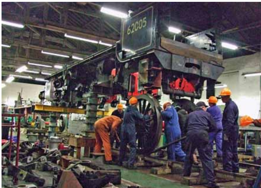
The first of the driving wheelsets is pushed back under the K1 at Hopetown on 17 th February (Colin Smith)
