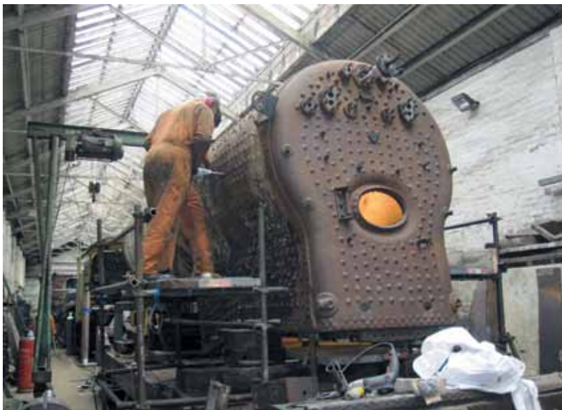
WCR staff drilling out old K1 firebox stays on 15 th February (John Hunt)
