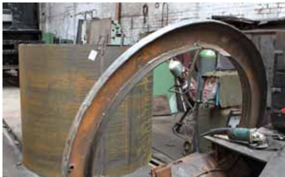
The repaired ring with the new smokebox wrapper behind (Paul Hutchinson)
