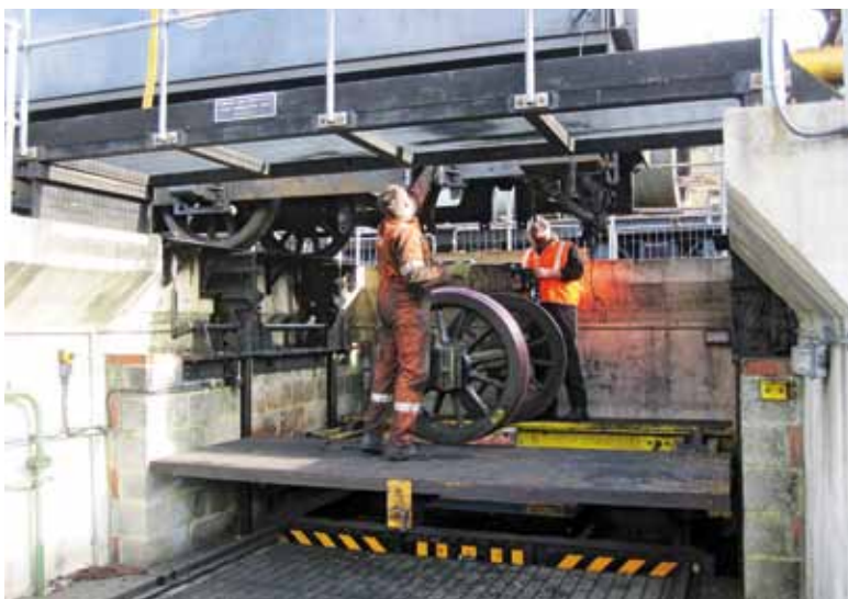
The Q6's leading tender wheelset is slowly raised back into the frames on the wheel drop at Grosmont on 24 th February (John Hunt)
