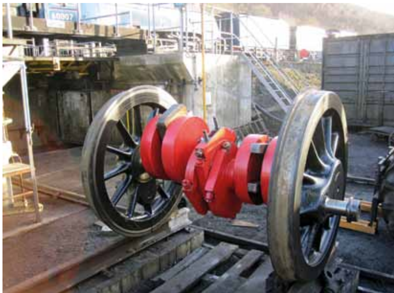
The J72's crank axle awaiting the refurbished axleboxes at Grosmont on 24 th February (John Hunt)
