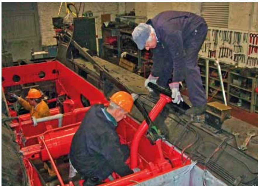
Allan Wilson and Steve Hyman attach a filler pipe to the new K1 sandbox, whilst Nigel Hall continues with frame painting at Hopetown on 3 rd March (Colin Smith)
