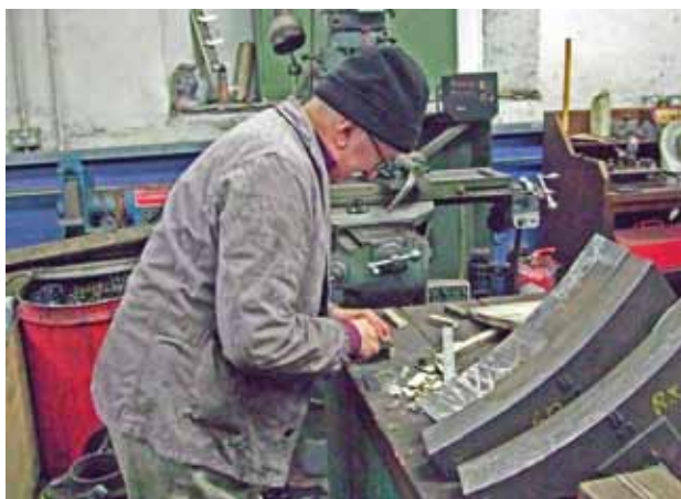
Martin Lloyd prepares some felt strips for the K1's coupling rods on 3 rd March; these rub on the journals and retain oil for lubrication (Colin Smith)
