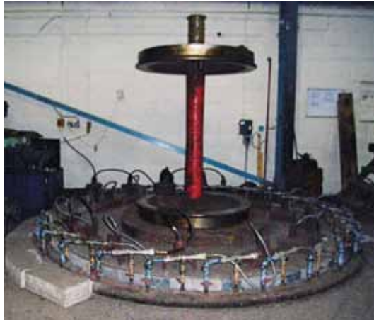
One of the K1 tender wheelsets receives a new tyre at Buckfastleigh on 15 th February (Neal Woods)
