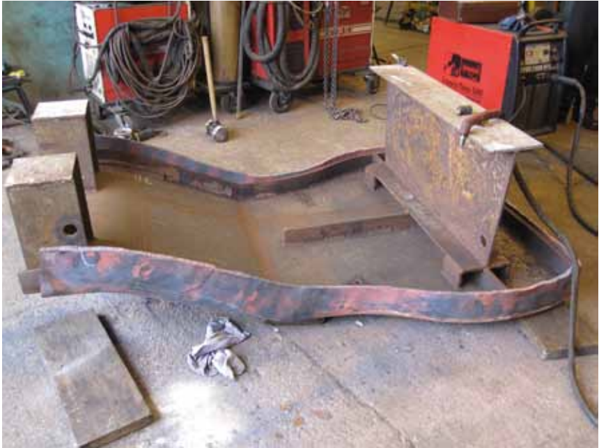
The new copper tubeplate surrounding the steel former on 6 th April and awaiting trimming (John Hunt)
