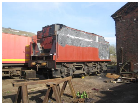
Contrasting views of the tender at Carnforth; on the left the old paintwork is rubbed down (Paul Hutchinson), whilst on the right the tender has received red primer (John Hunt)
