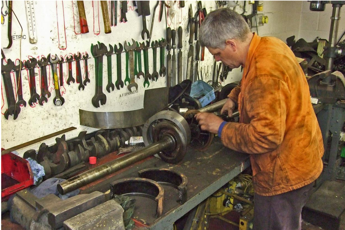
Richard Pearson fitting a new valve ring to the Q6 valve head at Grosmont on 28 th February; the broken one is in the foreground (Colin Smith)
