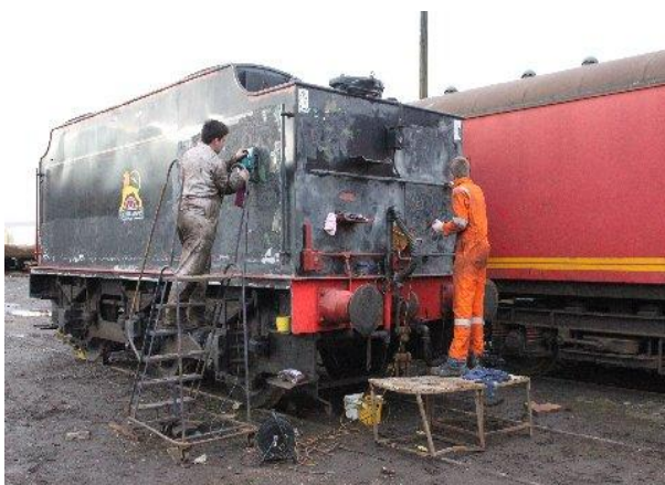
Contrasting views of the tender at Carnforth; on the left the old paintwork is rubbed down (Paul Hutchinson), whilst on the right the tender has received red primer (John Hunt)
