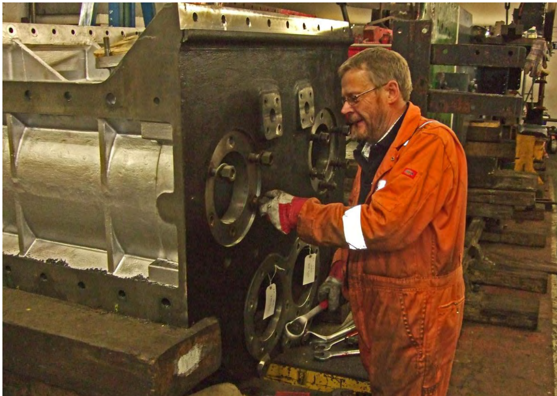
Andy Bell works on the cylinder block on 29 th November (Colin Smith)
