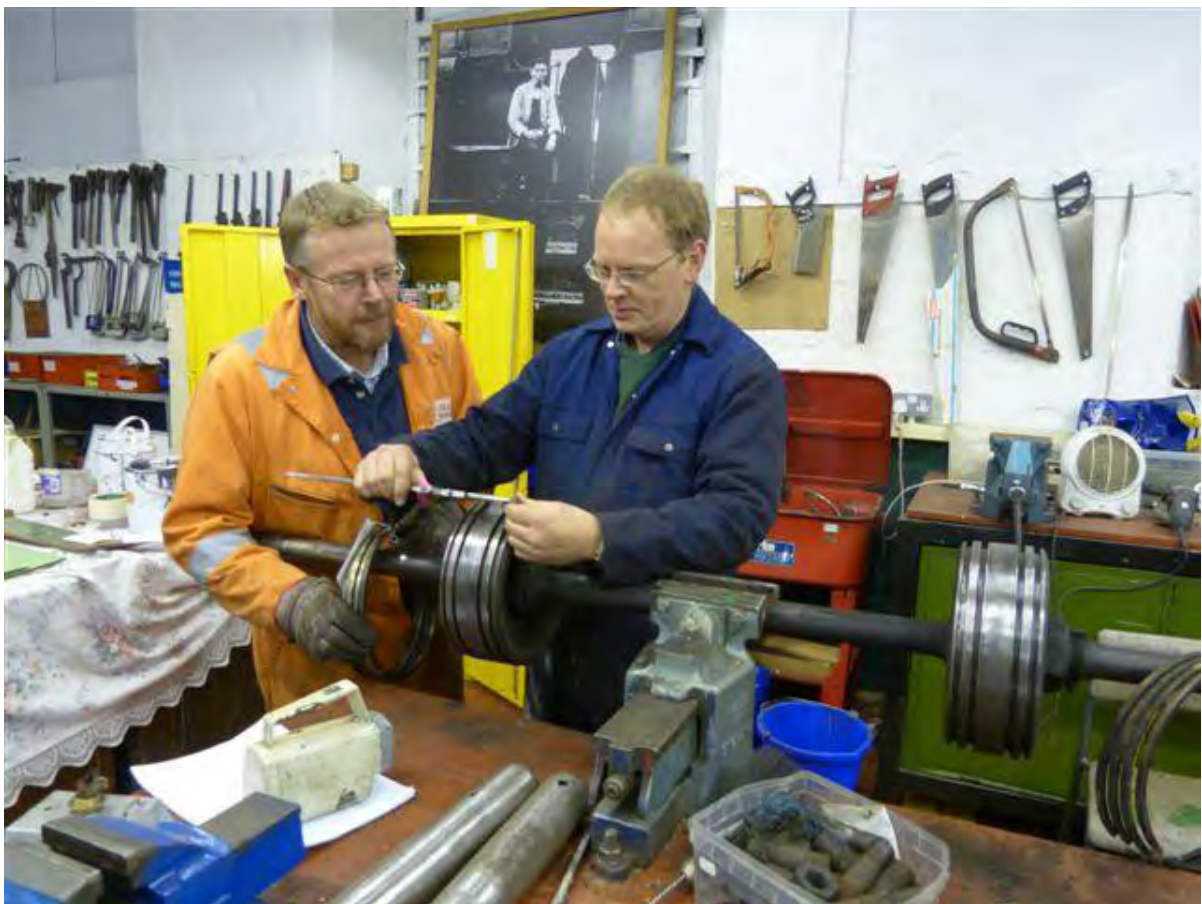
Andy Bell and Darrin Crone working on the K1 valve heads (Terry Newman)
