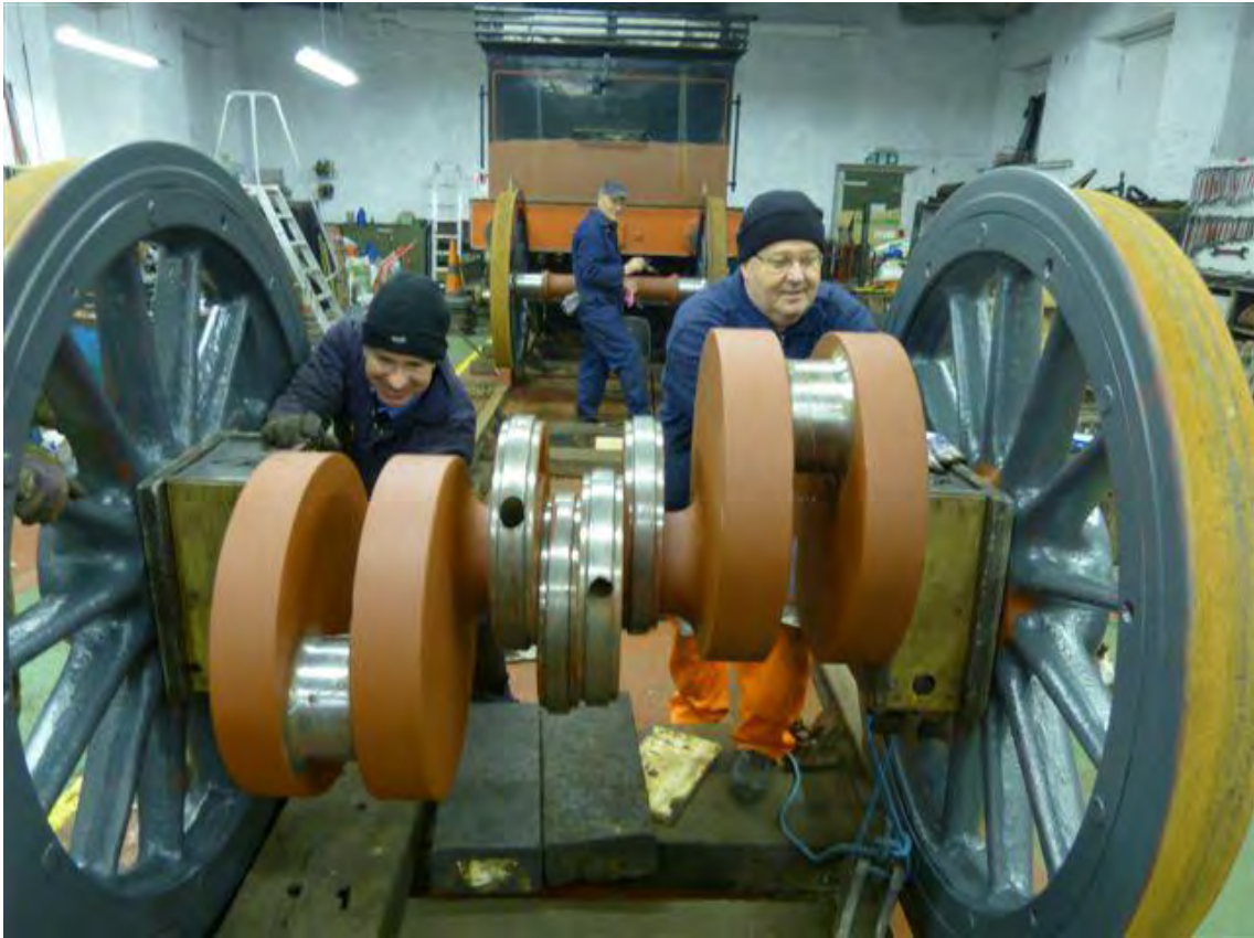
Steve Hyman and Nigel Bill (the new Hopetown caretaker) check the axleboxes on the J27 crank axle on 29 th November; in the distance Colin Bowman paints one of the wheelsets (Terry Newman)
