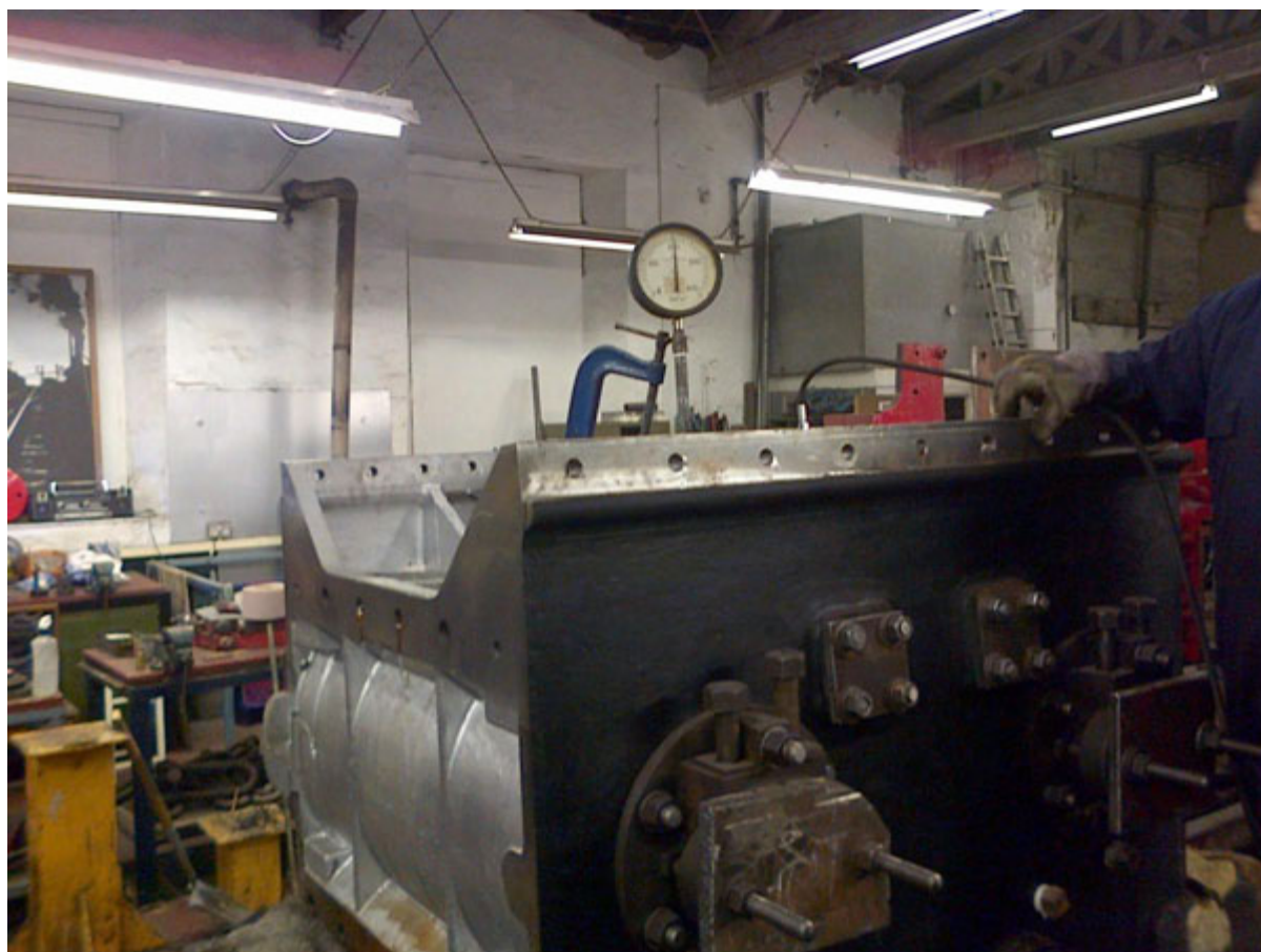
The cylinder block undergoing hydraulic testing on 8 th April (Rowland Bingham)
