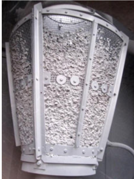
The K1's smokebox spark arrester almost completely clogged up on arrival back at Fort William depot on 23 rd May (John Hunt)
