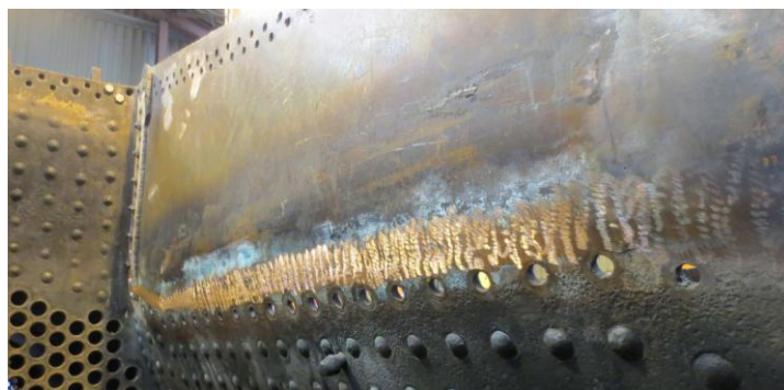
The LH copper side sheet in place on 19 th September (John Hunt)
