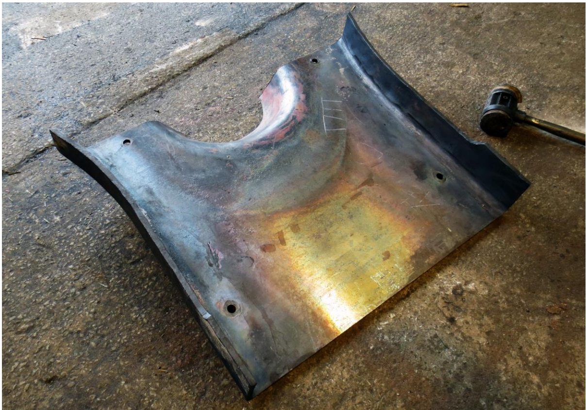
On the same day, the newly formed copper lower doorplate prior to fitting (John Hunt)
