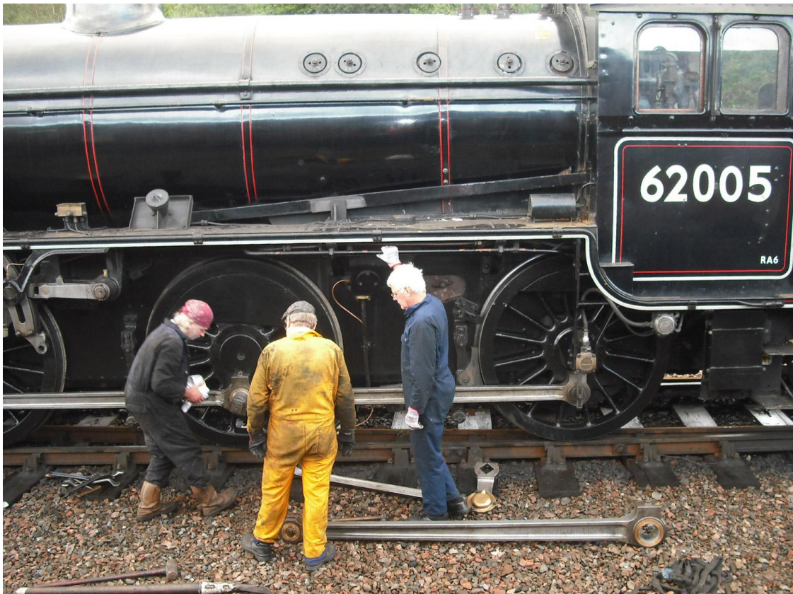
Paul Hutchinson, Nigel Hall and Dave Donegan refitting the connecting rods at Fort William on 21 st September (John Midcalf)
