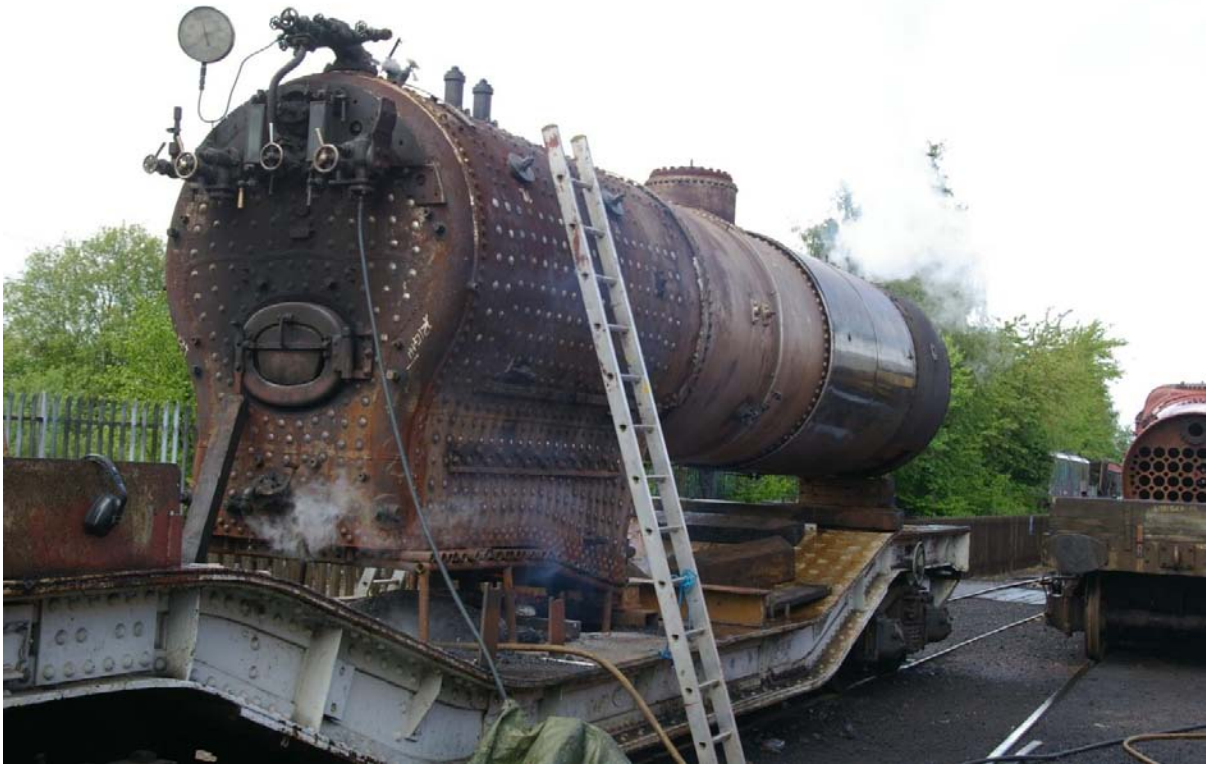
The Q6 boiler in steam for the insurance company inspector at Crewe on 13 th May (Chris Lawson)
