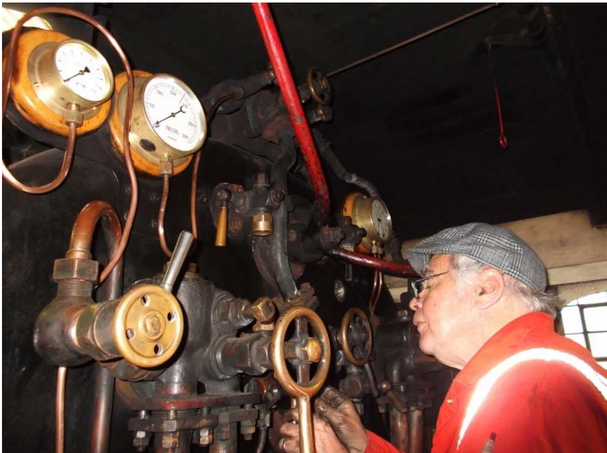
Mike Oliver, after completing the valve overhauls, has fitted the cab gauges, returned from overhaul from BKW Instruments, on 11 th March (Darrin Crone)
