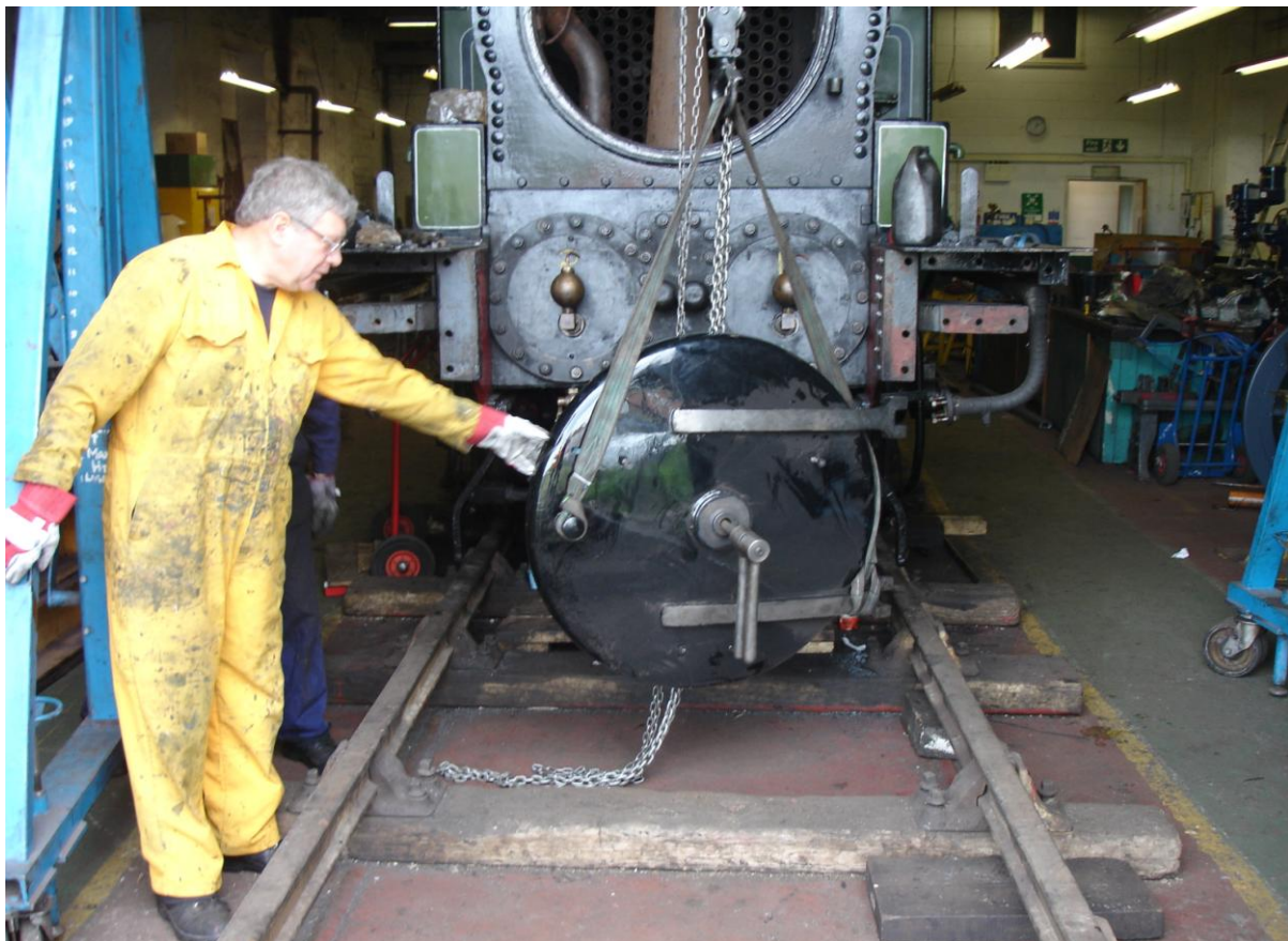
Nigel Hall guides the smokebox door ready for refitting (Fred Ramshaw)
