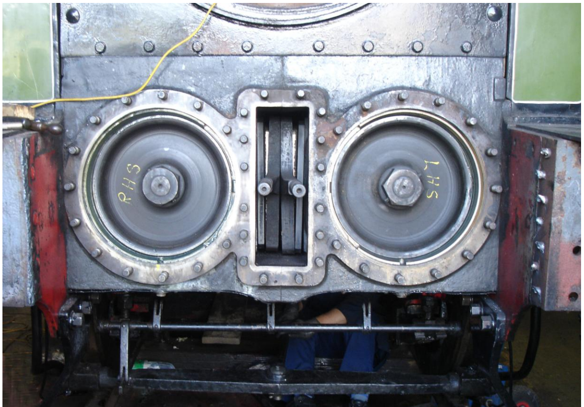
Both liners in, and pistons refitted showing, in between, the two slide valves (Fred Ramshaw).
