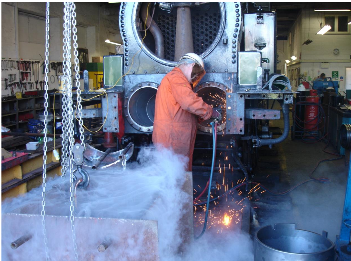
With the new liners cooling in a bath of liquid nitrogen, the cylinder bores are prepared for the liners to be slid in (Fred Ramshaw)
