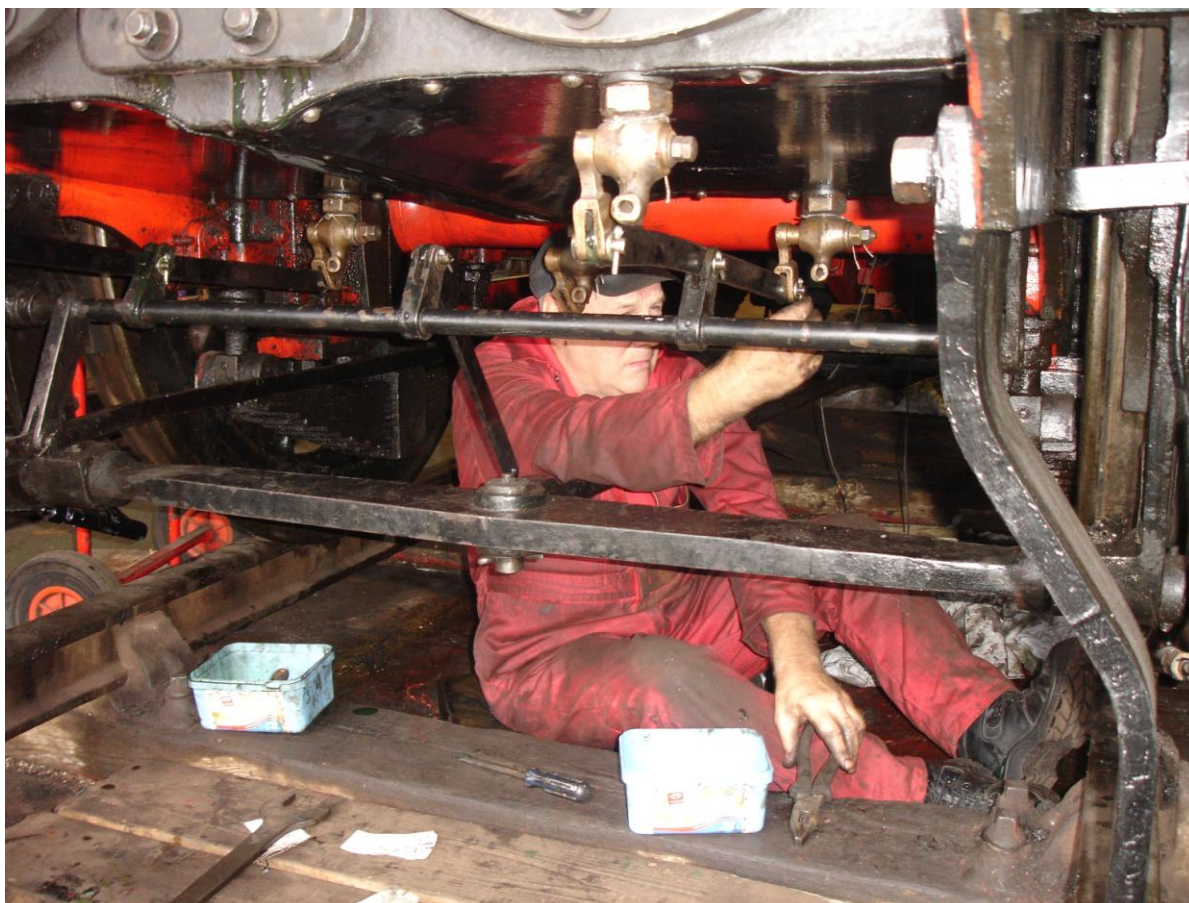
Steve Gibson refits the cylinder drain cocks (Fred Ramshaw)
