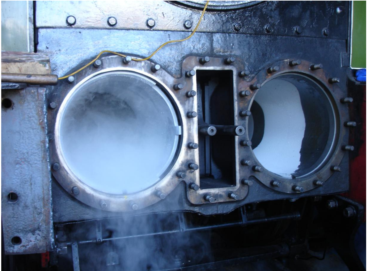
The RH liner in situ and cooling down (Fred Ramshaw)
