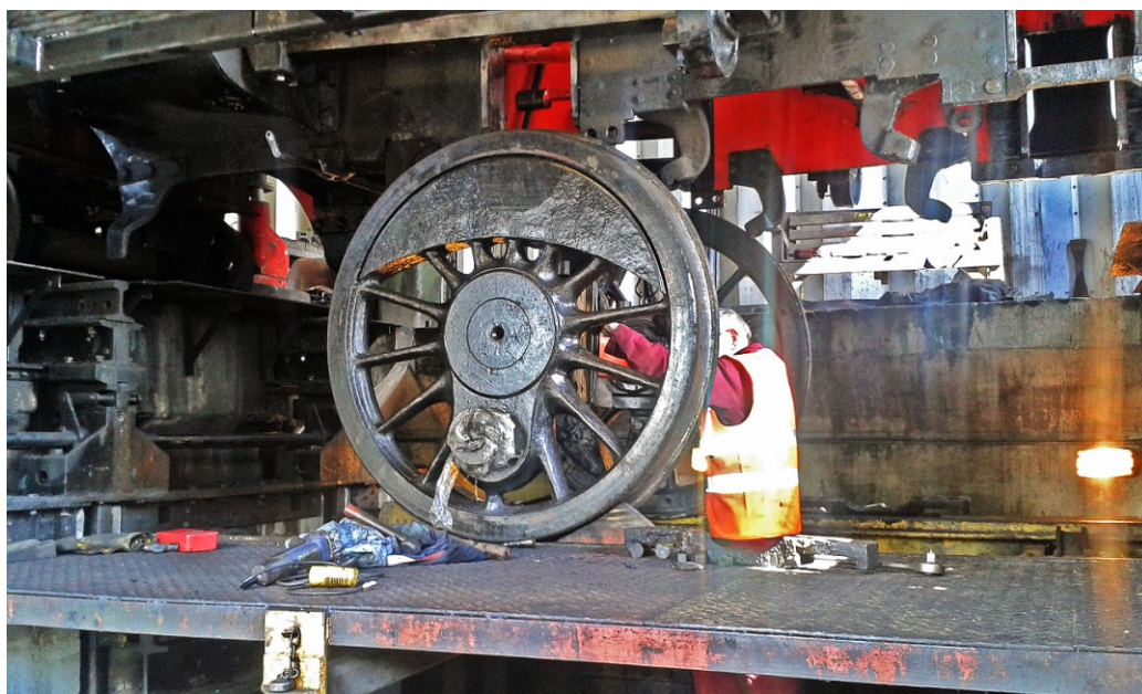
Lowering out the leading wheelset on the Grosmont wheel drop on 9 th May (John Hunt)
