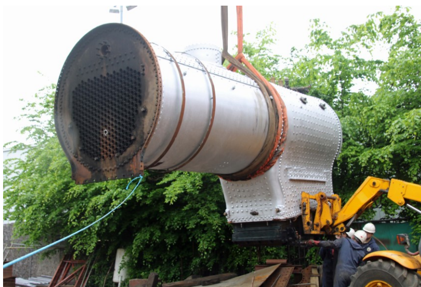
The boiler lift on 17 th May for trial fitting of the ashpan (Dave Pennock)
