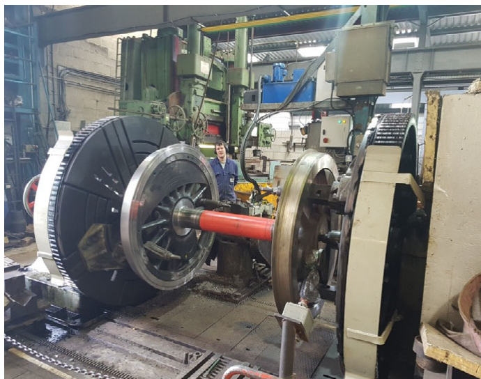
Left: Q6 the new front tubeplate in 2005, flue tube positions top (Dave Pennock) Right: Profiling of the new tyres at the South Devon Railway in July 2017 (Paul Pridham, SDR)
