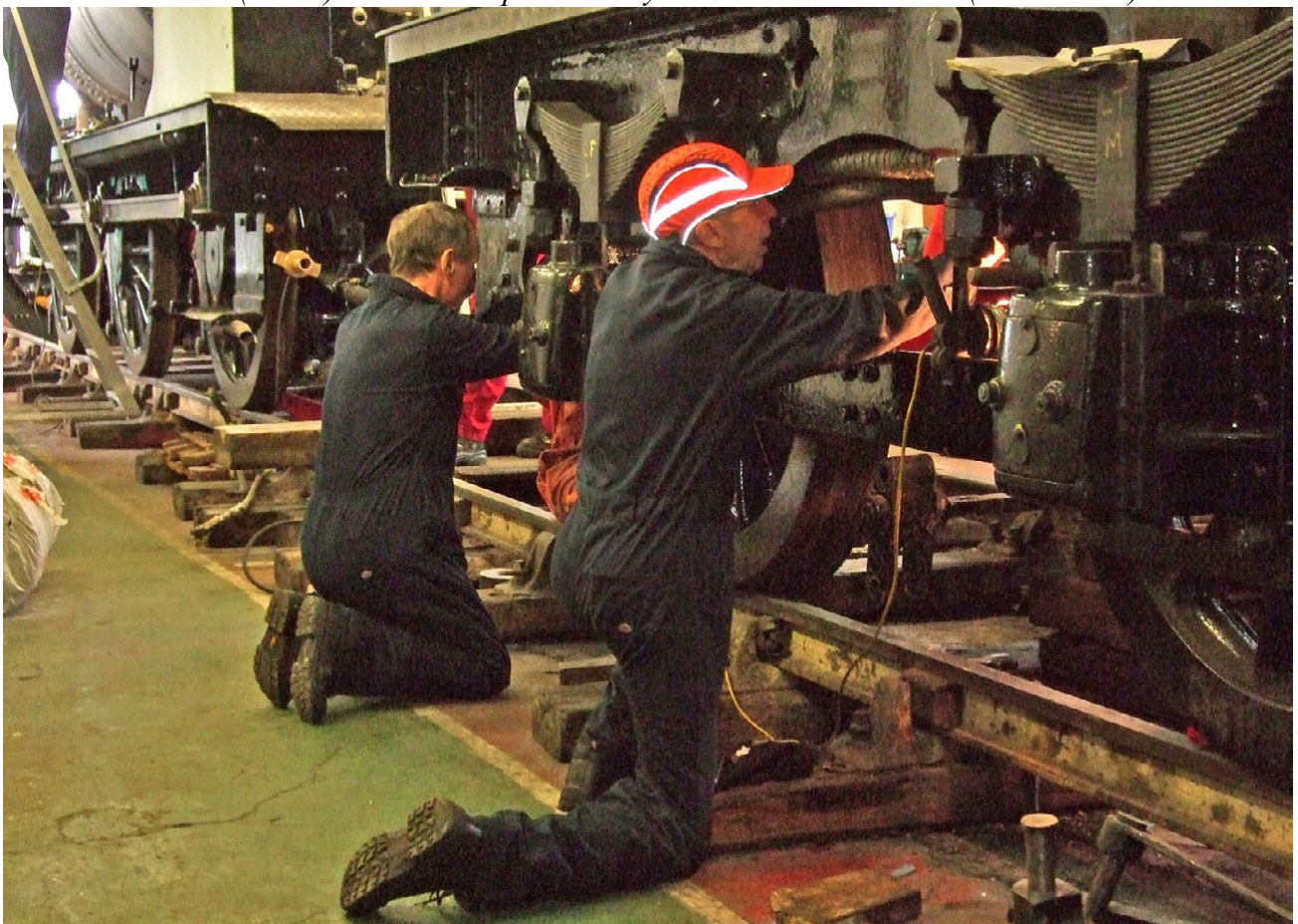
Work continuing on the J27 overhaul at Hopetown on 20 th July, with Harry Sams working on the boiler (above) and Les Harper and Roy Marshall on the tender (Colin Smith)
