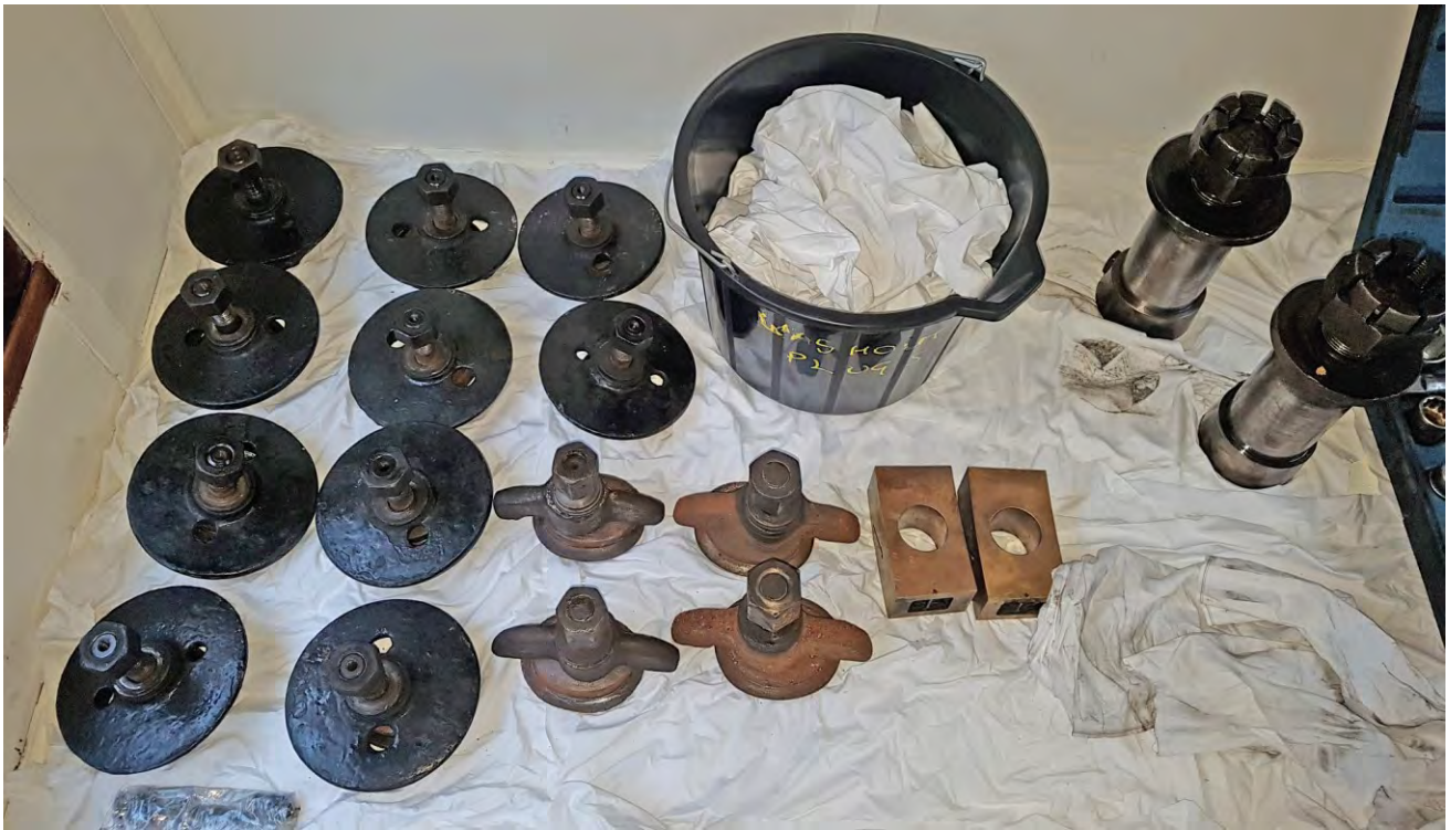
On the left the cleaned up boiler mud hole and washout doors, the two die blocks in the middle and the two little end pins on the right (Rowland Bingham)
