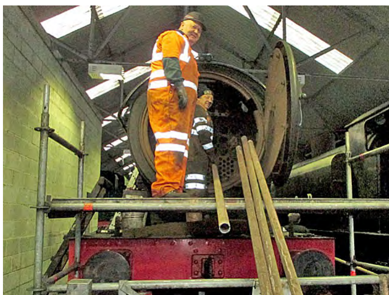
L. Trevor Wilford with a windy chisel collapsing the small tubes at the smoke box end (Nigel Hall) and R. Nigel Bill and Andrew Bullivant removing the last small tubes from the Q6 (Ian Pearson)
