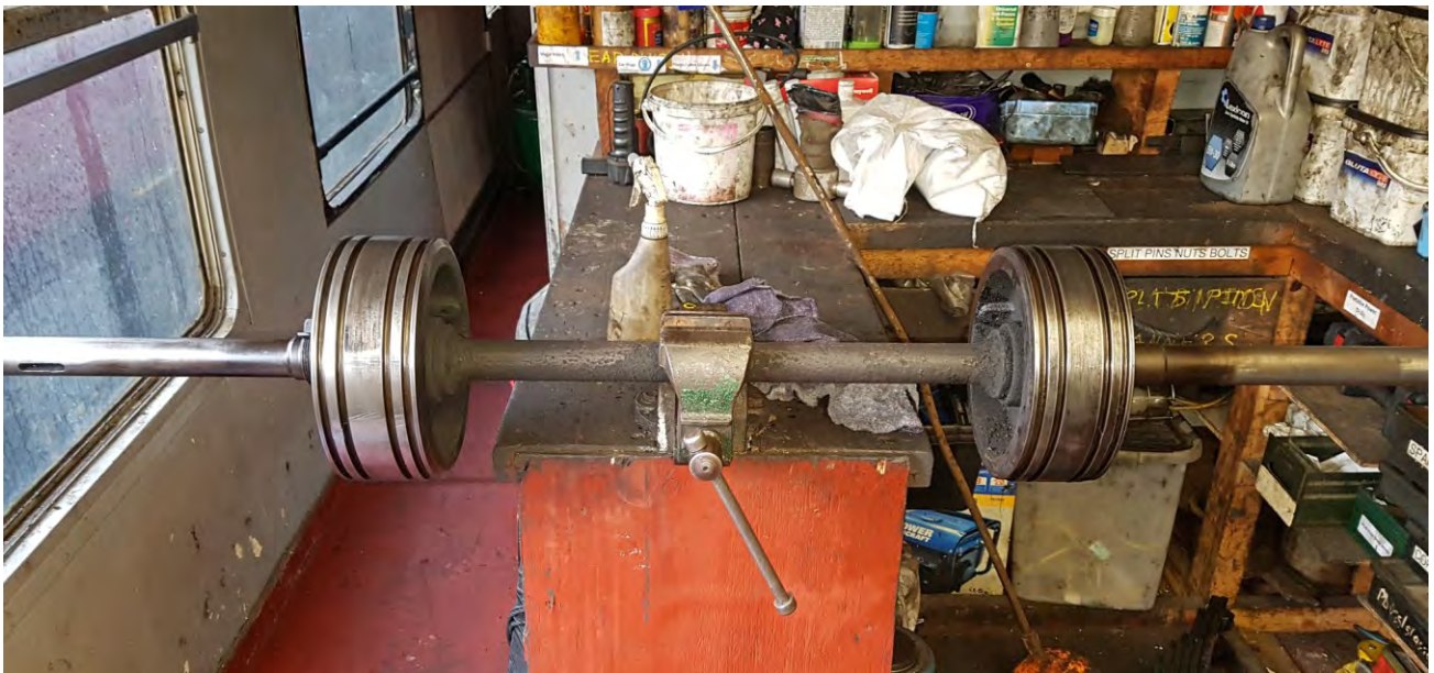
First to be removed, whilst the engine was still hot from its journey from Fort William, were the piston valves: here one of the valve rods and heads is cleaned up in the support coach workshop area (Rowland Bingham)
