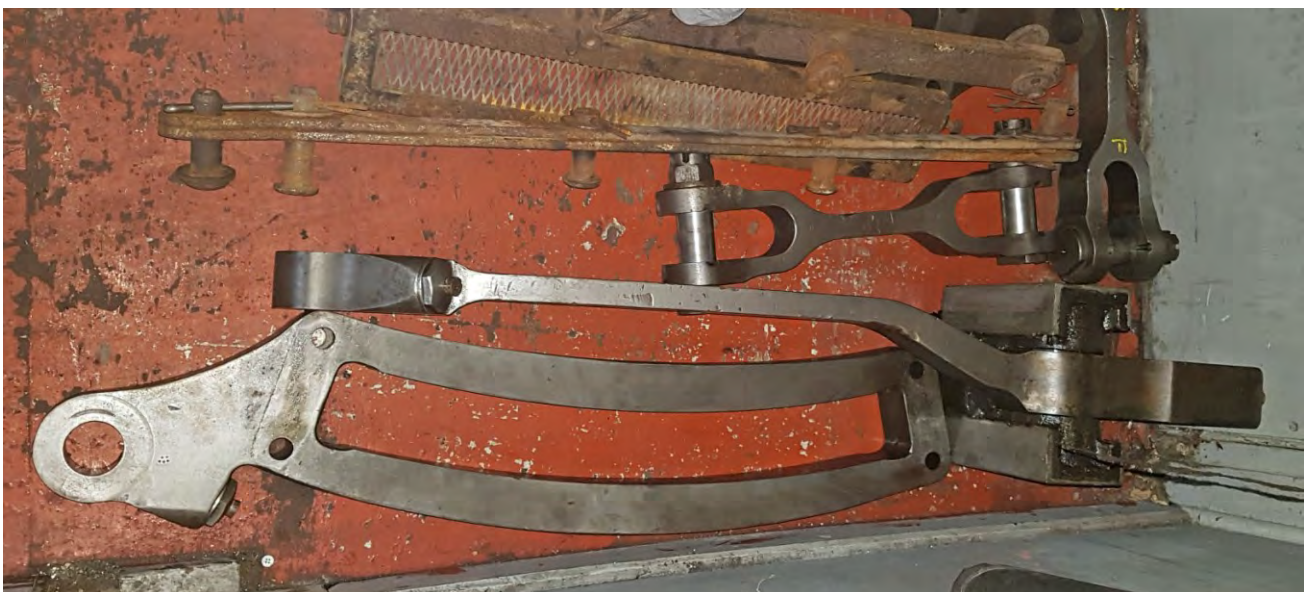
Also removed, and seen here, were the expansion links, combination levers and union links to be checked for wear, and refurbishment if necessary (Rowland Bingham)
