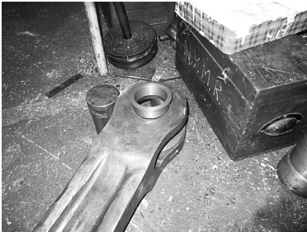
Q6 gradient pin bush and packing ready for pressing on 10 th January (Ian Pearson)
