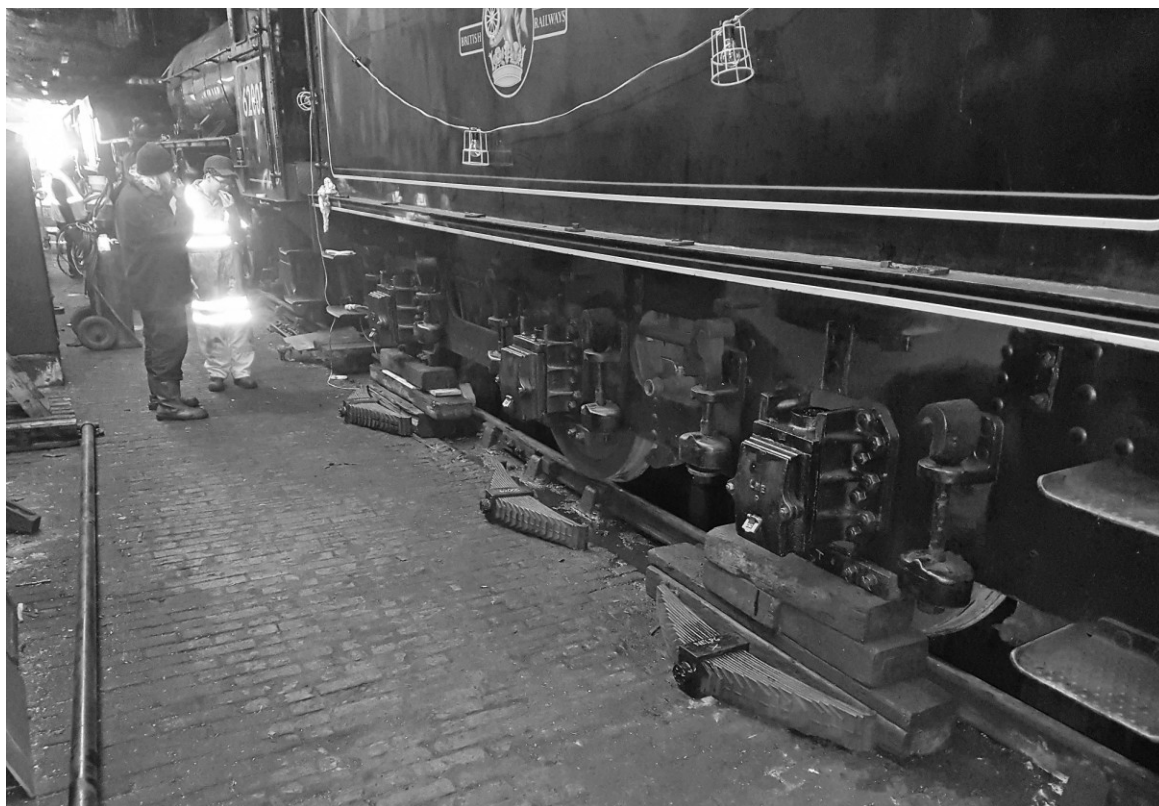
The K1's tender jacked up with the springs removed to allow examination of the axleboxes.
