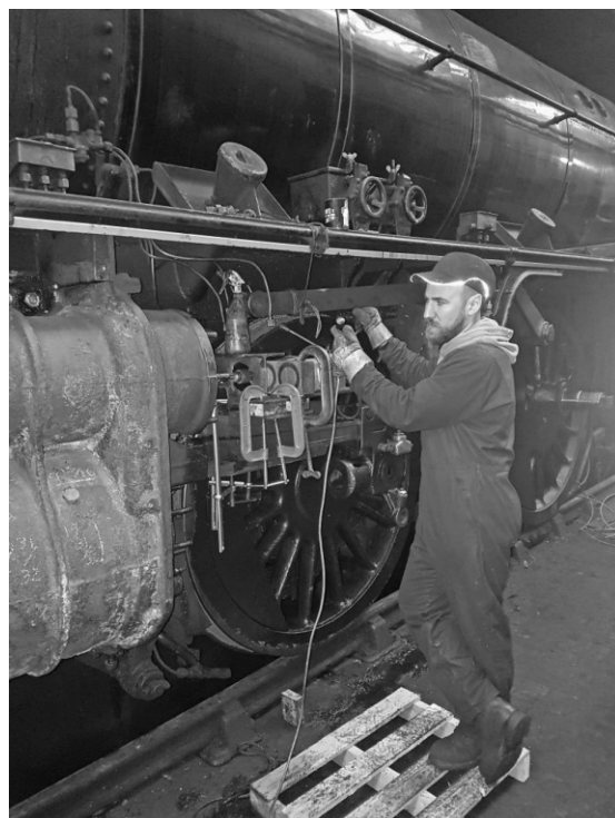
Angie Buxton with one of the K1's pistons and (right) Chris Henwood honing the K1's left rear piston valve liner (all Rowland Bingham)
