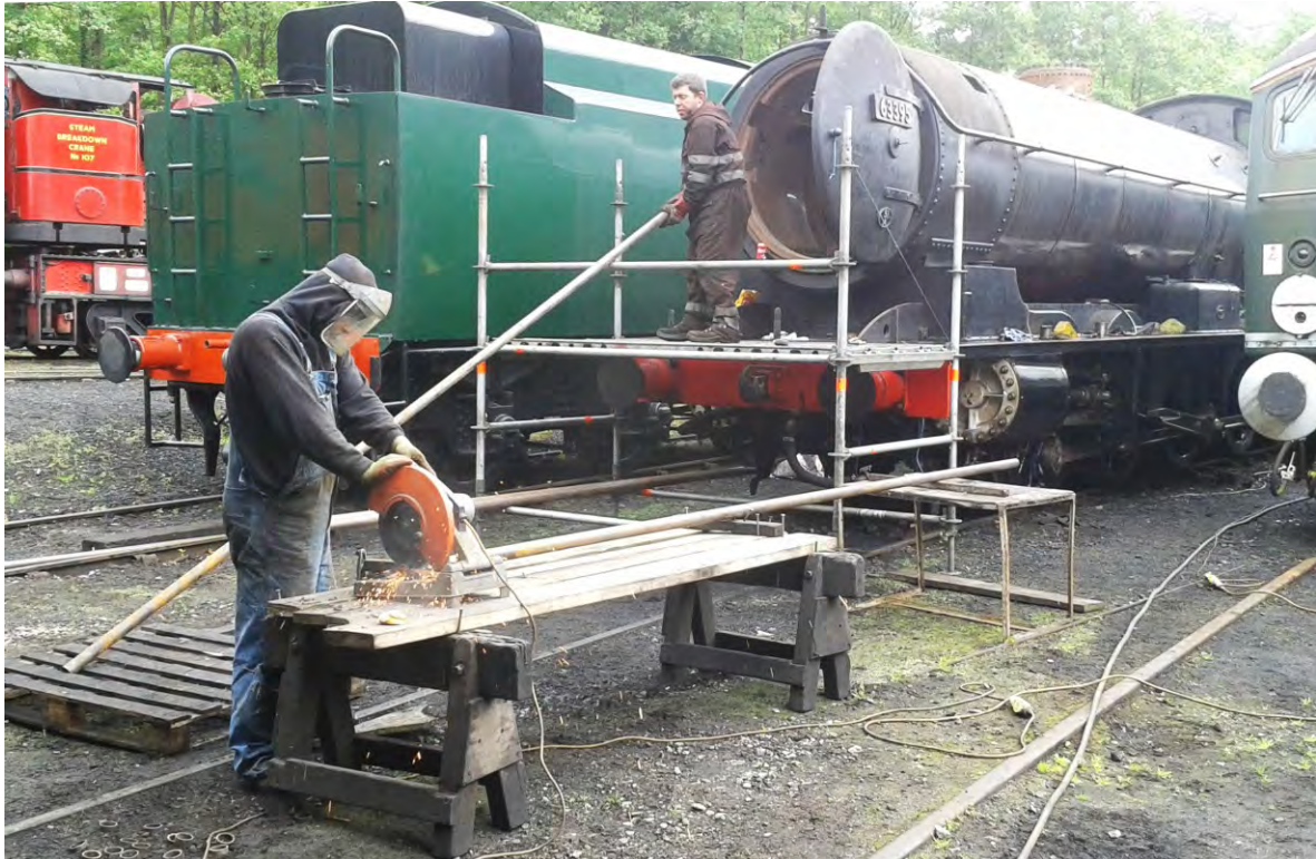
NYMR staff cutting to length and fitting the small tubes on 6 th June (Bill Dobson)
