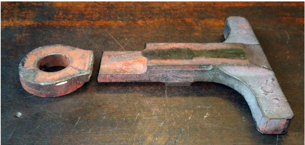
Another unforeseen problem was this broken regulator pilot valve, pictured on 28 th August (Barney Casey)
