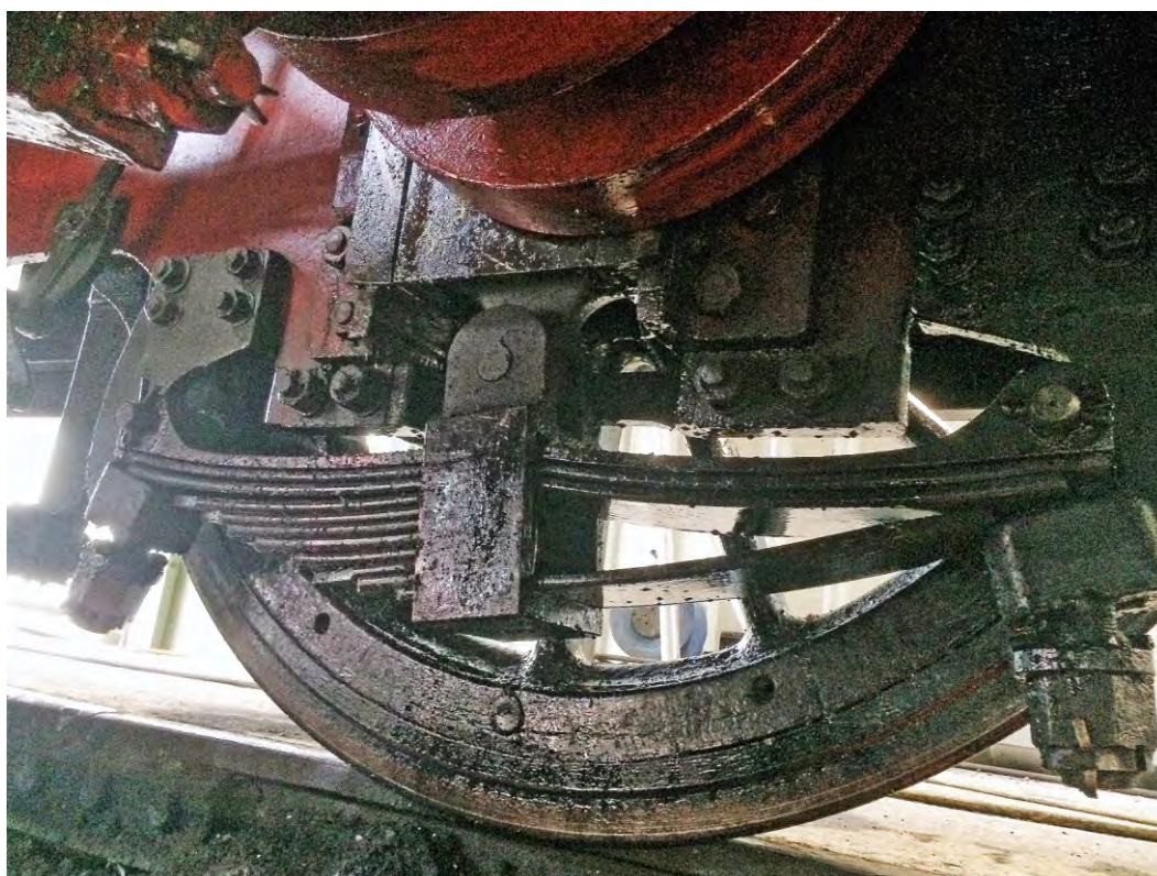
A shattered driving wheel spring on the J27 on 29 th August; 7 of the 11 leafs have completely disappeared, lying between the tracks west of Constable Burton! (John Midcalf)
