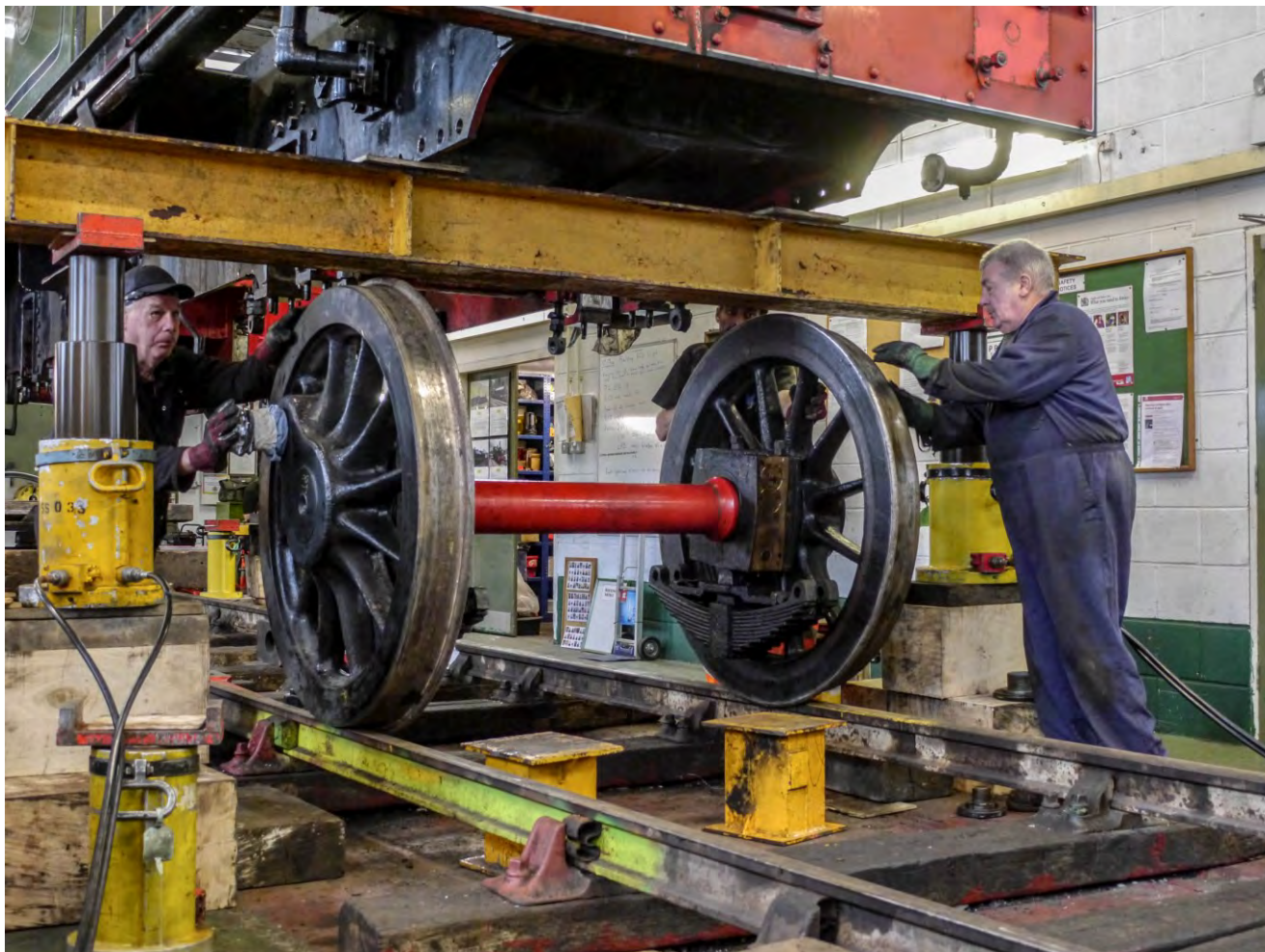
Steve Gibson (l) and Harry Sams roll out the J72's trailing wheel set (Peter Giroux)
