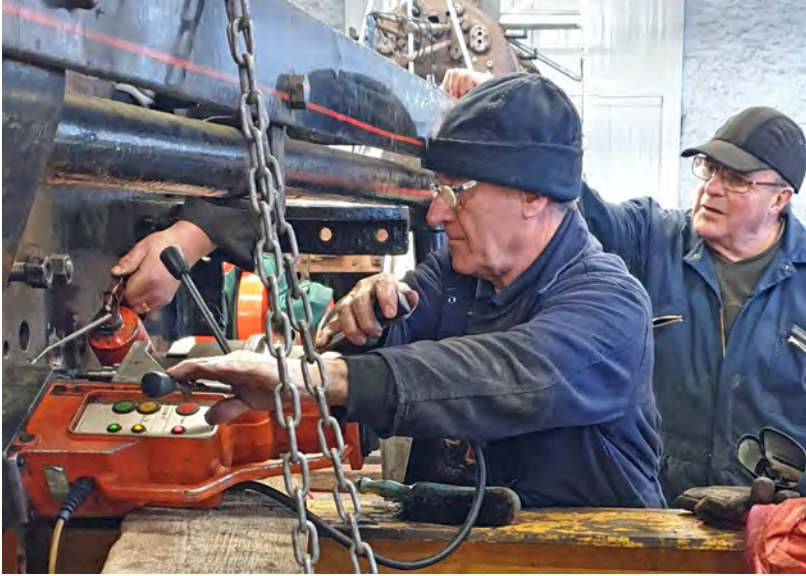
Machinists Arthur Jenkins and Maurice Bell with the magnetic drill which was recently repaired by Bill Dobson. The hand on the left pouring coolant onto the bit belongs to Ed Bolam. The fitted bolts securing the cylinder block are drilled, tapped and the extractor made by Maurice is then screwed into the countersunk end of the fitted bolt. By tightening the nut on the extractor the fitted bolt can be drawn out (Nigel Hall)
