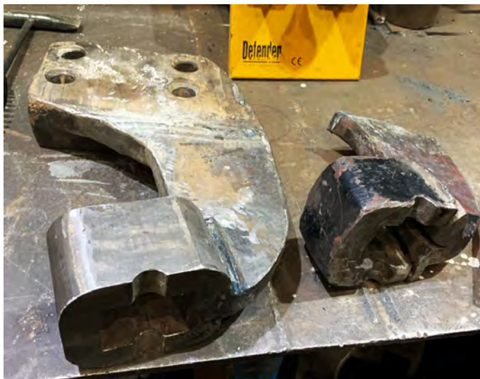
The broken spring hanger on the right and the new one made by Doug Foster and Nick Simpson, and machined by Owain Samuel.
