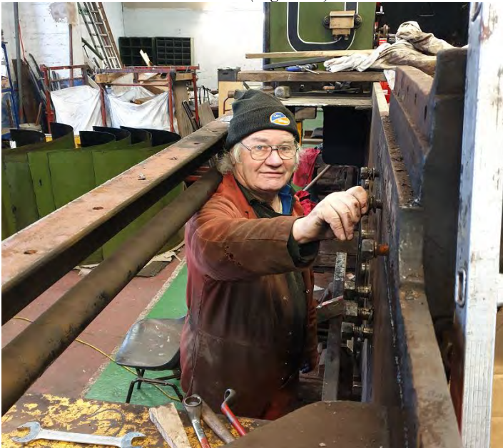
Tim Williamson replaces the angle iron nuts on the studs after removal of the J72 running board (Nigel Hall)
