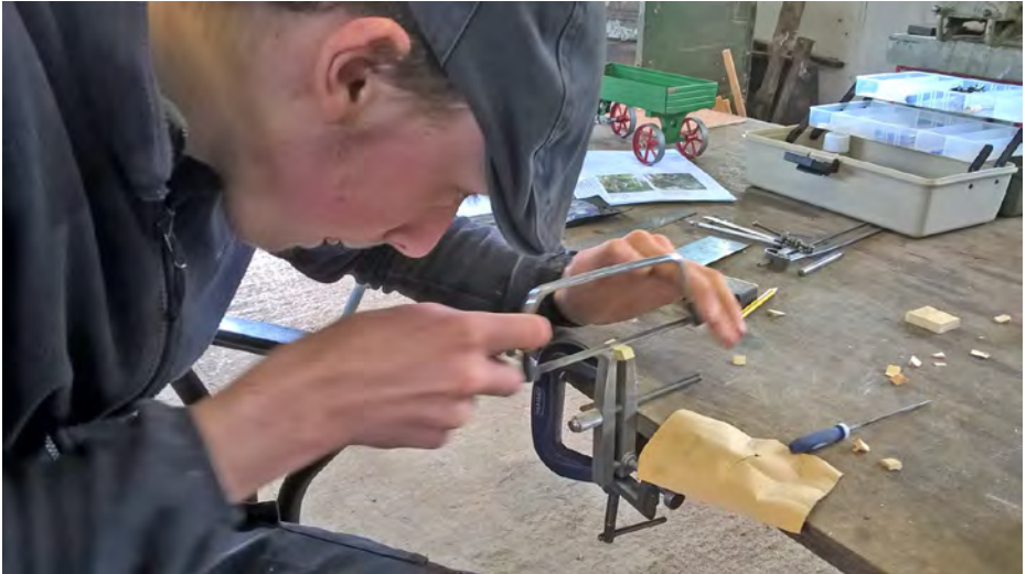
Finlay using the toolmaker's clamp to carefully cut the wheel segments.
