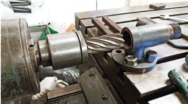
The Q6 steam reverser valve being machined at Ian Storey's workshop.
