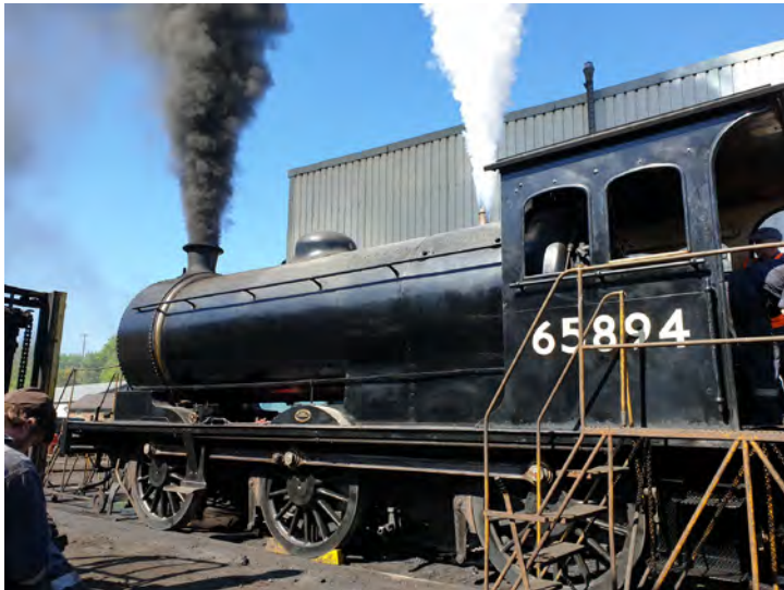
The safety valves lift on the J27 at Grosmont MPD on Monday 1 st June (Chris Henwood)
