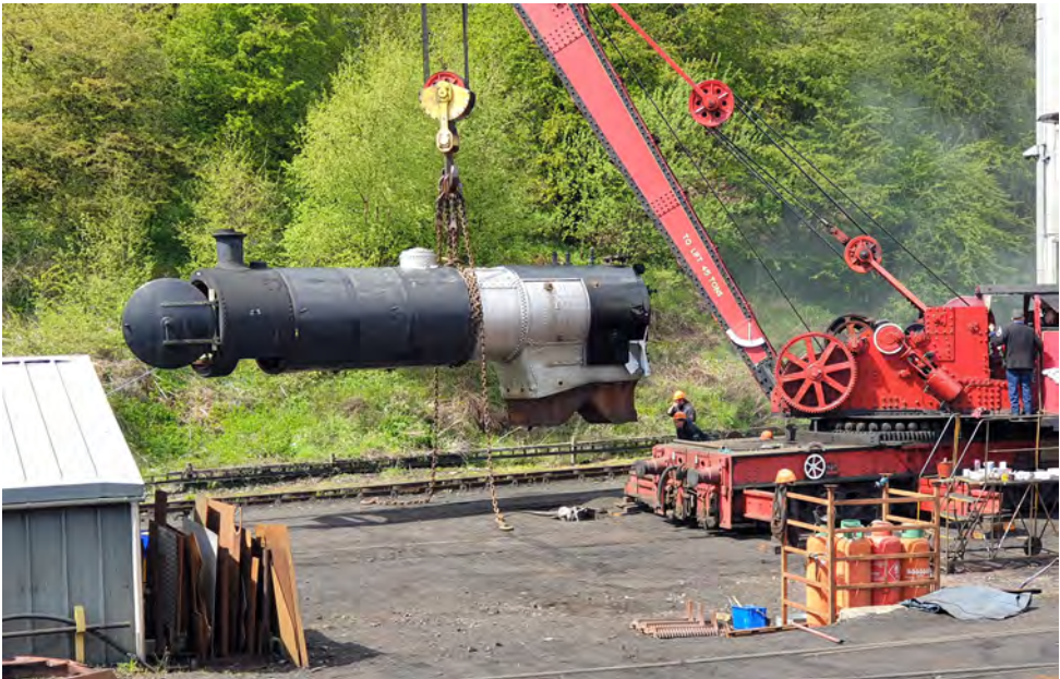
With Dave Cholmondley driving the crane under supervision from Charlie Dore, the Q6 boiler, complete with ashpan fitted, is lifted in readiness for reuniting with the frames on 12th May (Nigel Hall)
