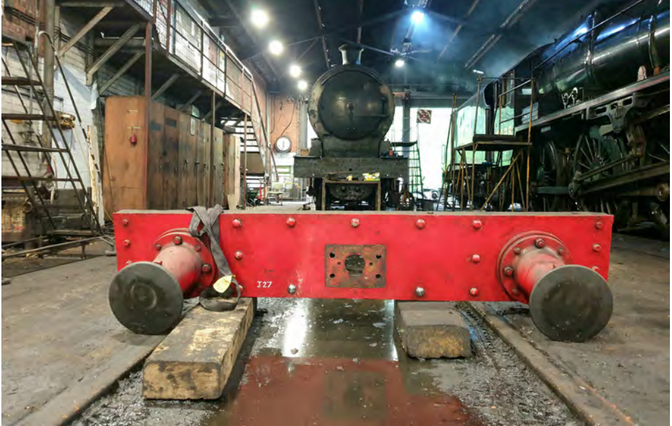
The J27 buffer beam ready to be reunited with the engine on 24th May (Chris Henwood)
