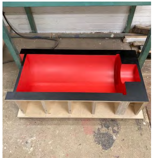
Two pictures of the J72 cylinder block pattern making (Dave Pennock / SLF)
