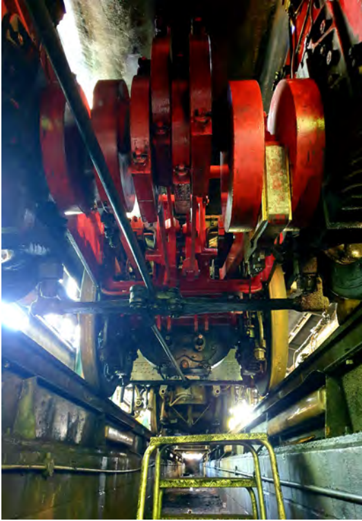
Viewed from the inspection pit, the eccentrics and big ends of the J27 on 4th June (Chris Henwood)
