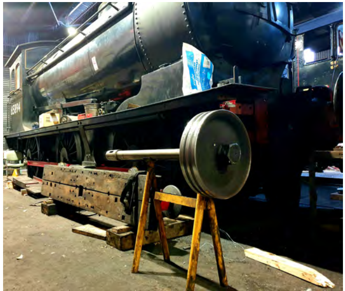
The RHS piston ready to be fitted after cylinder reboring on 1st May (Chris Henwood)
