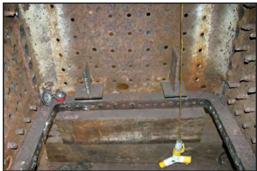
The front tubeplate (left) and the refurbished foundation ring refitted to the inner firebox (right) (Dave Pennock)
