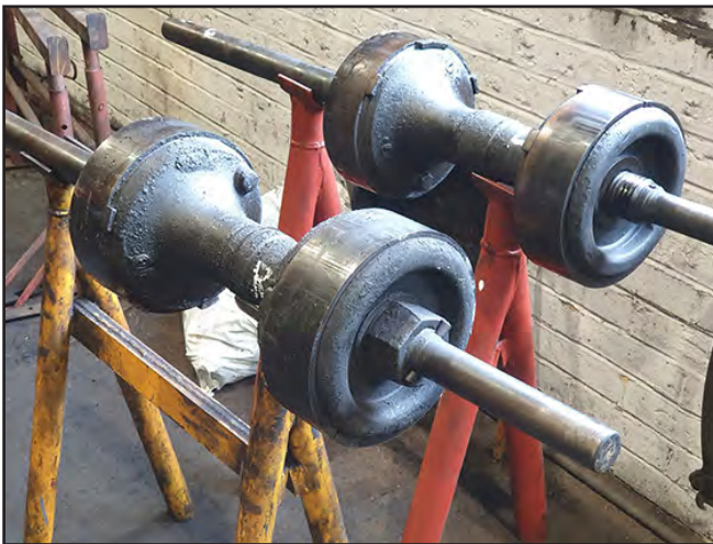
The Q6 valves removed on 12th July to check for damage or undue wear because of the perceived lack of lubrication (Nigel Hall)
