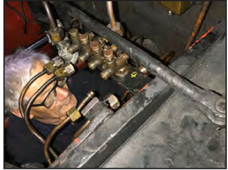
The non-return valves on the left, and Bill Dobson trial fitting them on 12th July (both Ian Pearson)
