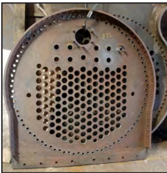
The front tubeplate (left) and the refurbished foundation ring refitted to the inner firebox (right) (Dave Pennock)
