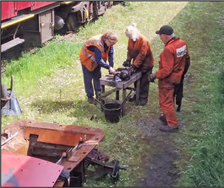
Angie, Lizzy and Steve cleaning the LH injector after removal, with the ashpan and centre section of the cab roof in the foreground (Paul Hutchinson)
