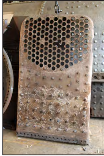
The backhead refitted, welded and clamped to retain the form of the firebox (left) and the copper tubeplate (right) (Dave Pennock)
