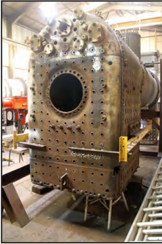
The backhead refitted, welded and clamped to retain the form of the firebox (left) and the copper tubeplate (right) (Dave Pennock)
