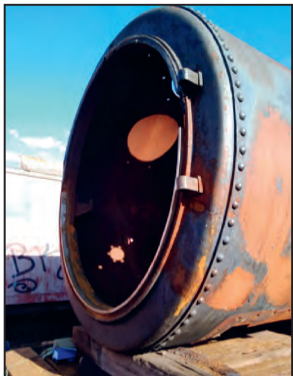
The partially refurbished smokebox door sealing ring (Paul Hutchinson)
