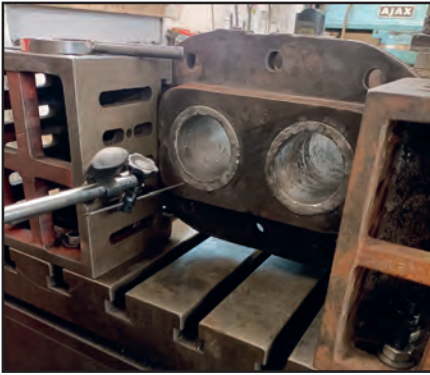
The J72 valve reach rod guide on the boring machine on 16th August (Neal Woods)
