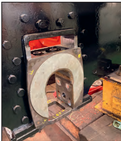
One of the refurbished J72 axle boxes successfully trial fitted on 27th September (Neal Woods)
