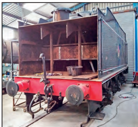
Left: The tender with the back of the tank and some of the baffles/bracing removed on 24th September Right: Jason Brown servicing one of the mechanical lubricators on 20th August (both Paul Hutchinson)
