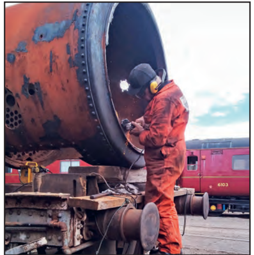
Steve Gibson working on the smokebox door ring on 20th August (Paul Hutchinson)
