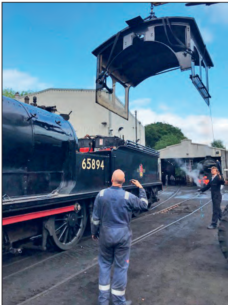
The J27 cab being refitted on 14th September (Ian Pearson)
