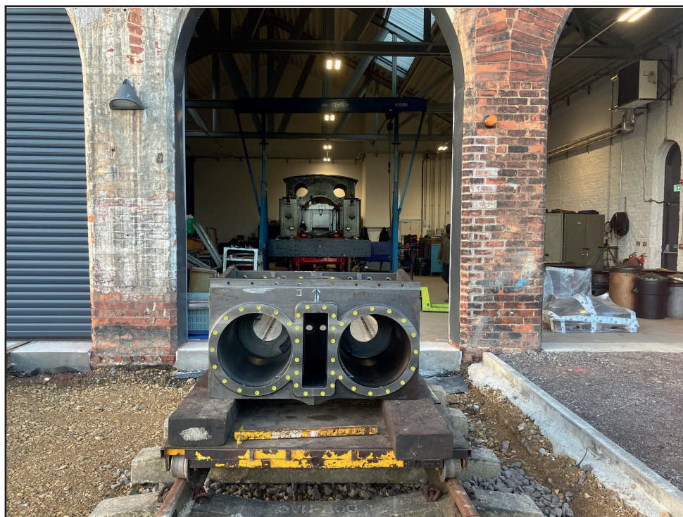
The J72's new cylinder block outside the 1861 shed following delivery from Dormer Engineering on 26th January. The next step is to hydraulically test the block before fitting it into the frames (Neal Woods)
