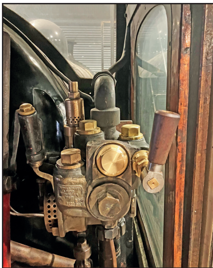
The P3's refurbished vacuum ejector showing the small ejector handle on the right and the large ejector handle on the left (Neal Woods)
