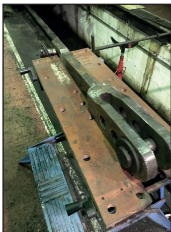
The link rod between the engine steam brake and tender weigh shaft after removal and cleaning for NDT testing on 14th November and the right-hand valve after cleaning by Trevor Wilford on the same day (both Ian Pearson)
