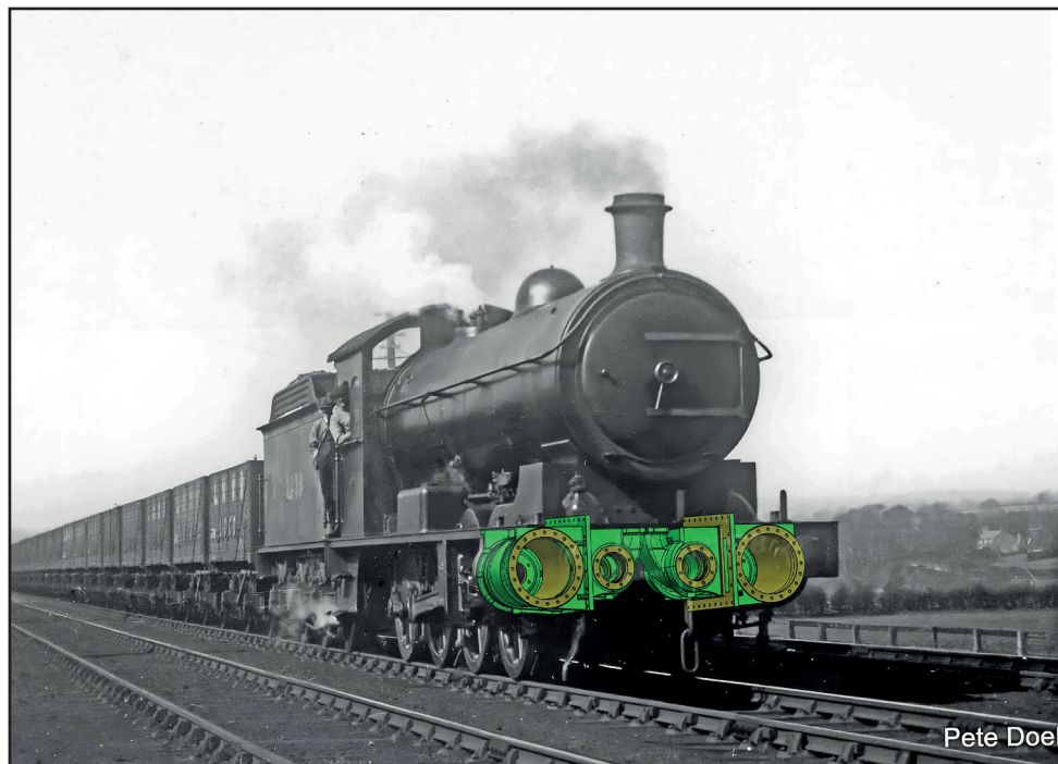
Using computer technology to good effect, two new 3D cylinders are superimposed on our Q6, as T2 2238, in this view taken at Low Fell.
