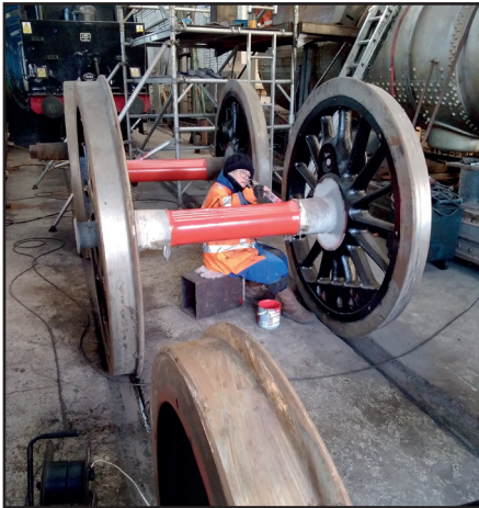
Angie painting the leading coupled wheelset axle. The photo also shows the wheels in black (not green) undercoat with the upturned boiler in the right background, and Angie preparing the pony wheelset for priming (taken from the K1's boiler) (both Paul Hutchinson)
