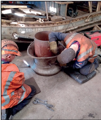
Steve Gibson peening one of the chimney liner securing studs after it had been warmed by Les Harper with the oxy gear, and Steve with the assembled chimney, liner and ejector exhaust ring/petticoat (both Paul Hutchinson)
