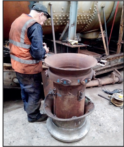
Steve Gibson peening one of the chimney liner securing studs after it had been warmed by Les Harper with the oxy gear, and Steve with the assembled chimney, liner and ejector exhaust ring/petticoat (both Paul Hutchinson)
