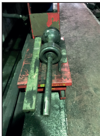
The link rod between the engine steam brake and tender weigh shaft after removal and cleaning for NDT testing on 14th November and the right-hand valve after cleaning by Trevor Wilford on the same day (both Ian Pearson)
