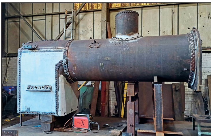
A view of the J72 boiler, now with the dome fitted, on 24th January (Dave Pennock)
