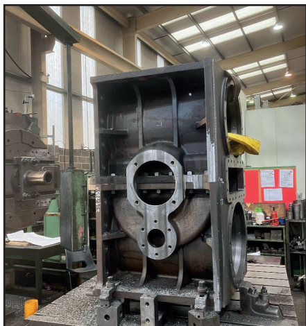
Left: looking at the top of the block, with the front on the right. The smaller orifice is the steam supply to the slide valves (in the middle front), and the larger orifice is the exhaust. Right: the bottom and rear of the cylinder block, with the holes for the valve spindles in the middle and, on the bottom, fore and aft, are the holes for the cylinder drain cocks (both Neal Woods)
