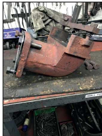
Left: the view into the dome showing the main steam pipe, with the boiler tubes below. Right: the 'J' pipe with the connection to the main steam pipe on the left and the regulator assembly area on the top right (both Ian Pearson)
