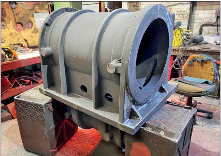
The new Q6 cylinder casting (Boro Foundry)
