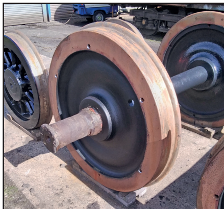
One of the tender tyres showing the countersinking (Paul Hutchinson)
