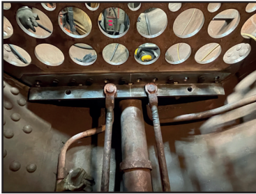
The new strap trial fitted (left) and the strap after welding (right) (both Paul Hutchinson)
