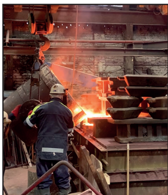
The molten iron being poured on 18th March and the finished casting (both Boro Foundry)
