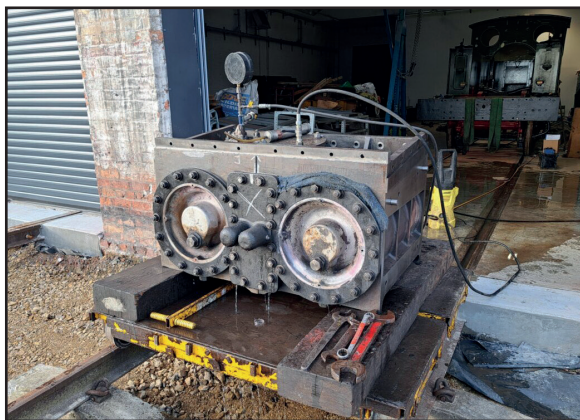
The new J72 cylinder block undergoing hydraulic testing (Ed Bolam)
