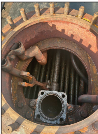
Left: the view into the dome showing the main steam pipe, with the boiler tubes below. Right: the 'J' pipe with the connection to the main steam pipe on the left and the regulator assembly area on the top right (both Ian Pearson)
