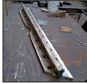
The new strap trial fitted (left) and the strap after welding (right) (both Paul Hutchinson)
