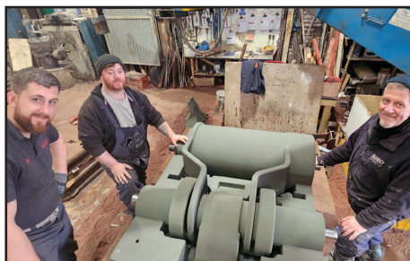
Three views of the mould showing its complicated nature and, hence, the high cost of production (all Boro Foundry)
