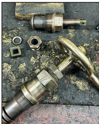
Left: the left-hand injector clack box parts after servicing on 9th February. Right: the new and old driver's seats, the latter being almost life expired (both Ian Pearson)
