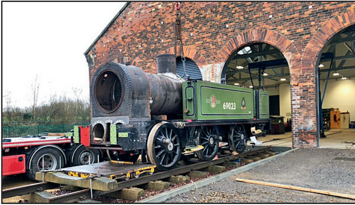
The boiler temporarily sat in the frames outside the 1861 shed on 22nd February (Ed Bolam)
