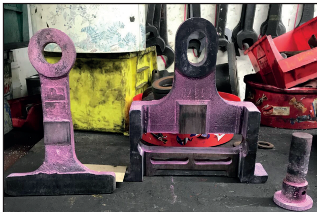
The regulator parts ready for NDT examination (Ian Pearson)
