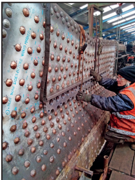
Angie Buxton with the new right-hand expansion bracket, held in place by stays, and Kenneth Morrison removing scale from roof stay threads (both Paul Hutchinson)
