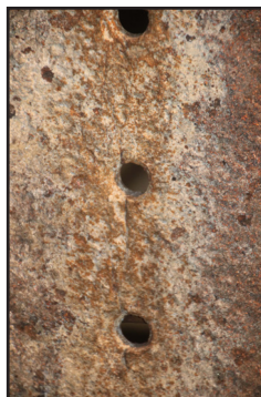
Left: the J72's left-hand side firebox expansion bracket highlighting the extent of metal loss around the fixing point. Right: grooves around a centre stay hole in the J72's throatplate (both Dave Pennock)
