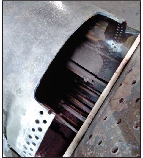
The bottom of the boiler barrel where it joins the throatplate showing the cracking on the left and the affected area cut out on the right on 5th January (both Paul Hutchinson)
