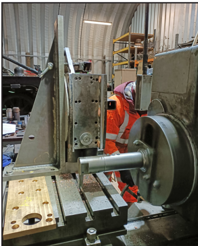
One of the J72 driving axleboxes being machined at NSEL on 25th January (Ian Storey)
