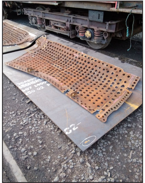
Left: James Grant putting the finishing touches to the foundation ring refurbishment on 20th January Right: The new and old firebox wrapper sides pictured on 21st December 2022 (both Paul Hutchinson)
