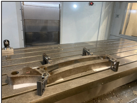
Left: The photo shows the KI's left-hand side expansion link on one of the Hass CNC milling machines being skimmed to remove waste
