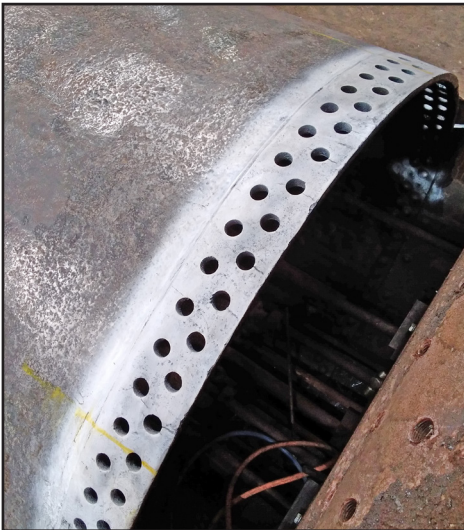
The bottom of the boiler barrel where it joins the throatplate showing the cracking on the left and the affected area cut out on the right on 5th January (both Paul Hutchinson)
