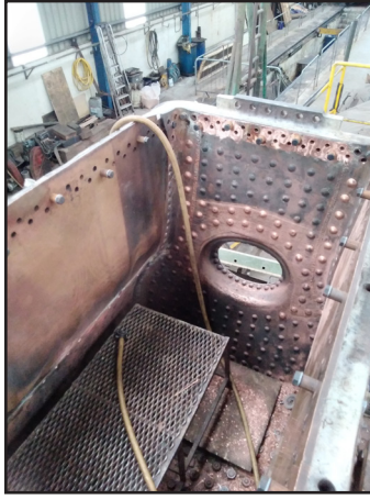
Three views of the boiler work: on the left, the backplate showing the new stays; middle, the new doorplate stays from the inside and the new copper side sheets; and right, the firebox awaiting the outer sheets, with the foundation ring in place (Paul Hutchinson)
