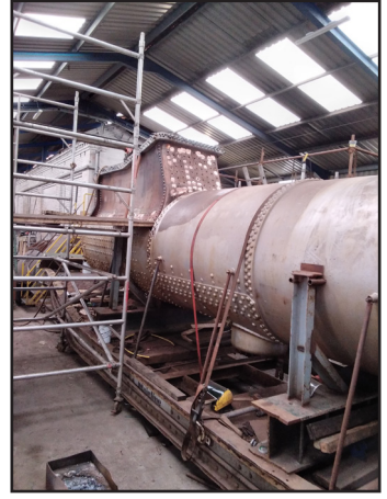
Three views of the boiler work: on the left, the backplate showing the new stays; middle, the new doorplate stays from the inside and the new copper side sheets; and right, the firebox awaiting the outer sheets, with the foundation ring in place (Paul Hutchinson)
