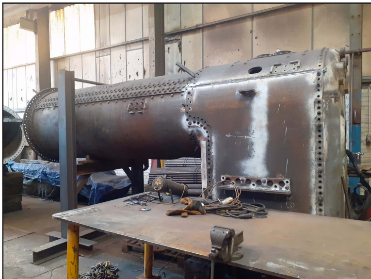
A view showing the left-hand outer side plate welded to the boiler crown (Dave Pennock)
