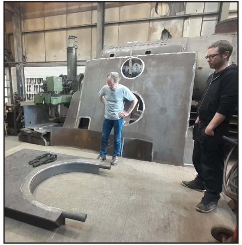
Left: the existing front throatplate to be replicated using a new former (Dave Pennock) Right: Roy Marshall (left) and Danny Dymott, NSEL (right) examine the steel throatplate former (Dave Pennock)
