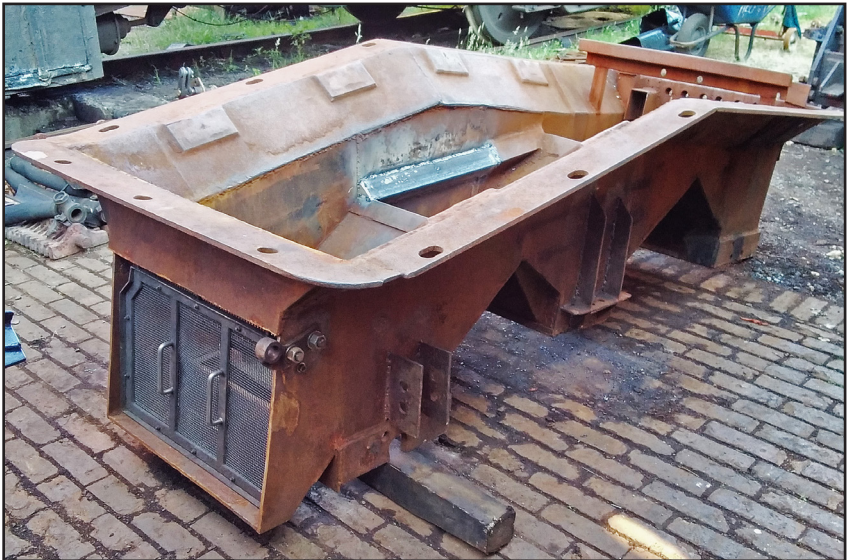
The refurbished ashpan minus damper doors (Paul Hutchinson)
