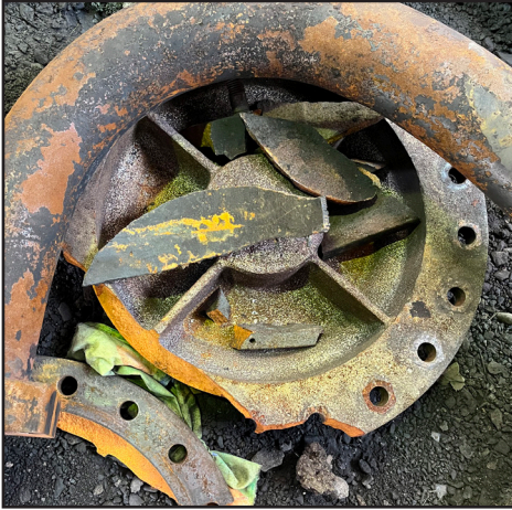
Left: nine of the broken parts of the cylinder and its front cover (John Hunt) Right: the external steam pipe dug out of the concrete (Ian Pearson)
