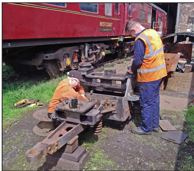
Angie Buxton and Chris Williams deep cleaning the pony frames (Paul Hutchinson)
