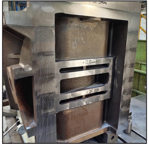
The right-hand cylinder before and after machining work (Neal Woods)
