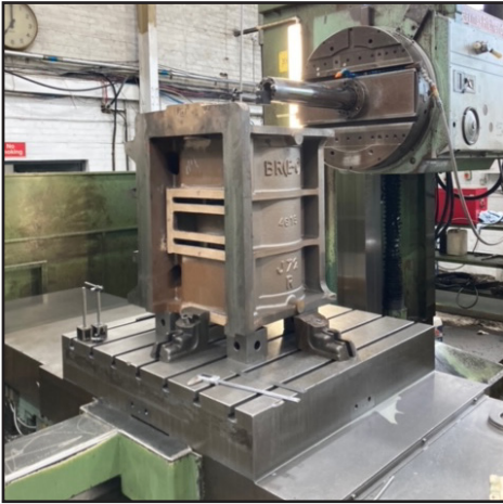
The right-hand cylinder before and after machining work (Neal Woods)
