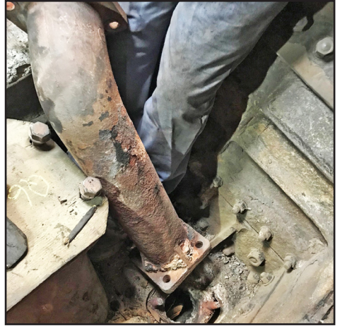
Left: nine of the broken parts of the cylinder and its front cover (John Hunt) Right: the external steam pipe dug out of the concrete (Ian Pearson)
