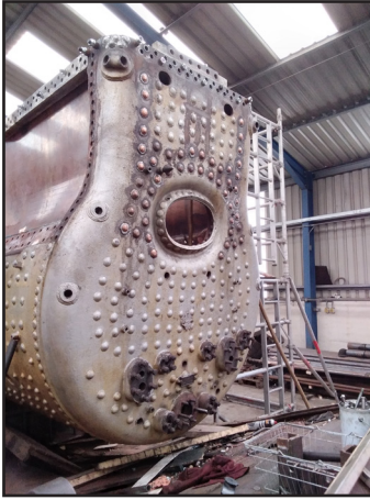
Three views of the boiler work: on the left, the backplate showing the new stays; middle, the new doorplate stays from the inside and the new copper side sheets; and right, the firebox awaiting the outer sheets, with the foundation ring in place (Paul Hutchinson)
