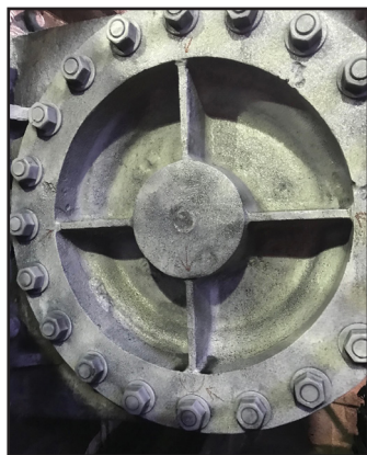
Left: the left-hand cylinder after successful MPI testing on 29th November.
