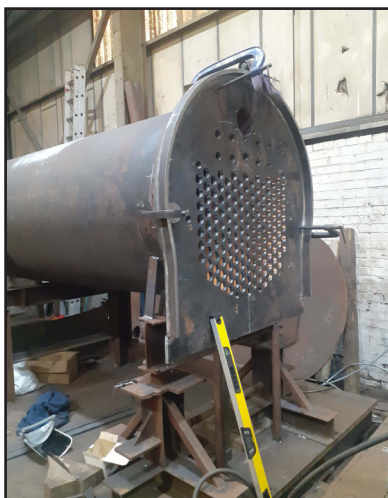
The new front tubeplate fitted to the boiler barrel on 1st November (Dave Pennock)
