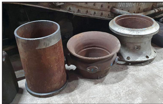
The new liner, ejector exhaust ring and chimney on 26th November (Paul Hutchinson)
