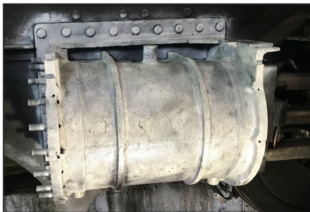
Left: the left-hand cylinder after successful MPI testing on 29th November.
