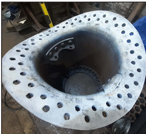
The upturned dome showing the boiler face cracks welded up and NDT tested on 1st November (Dave Pennock)
