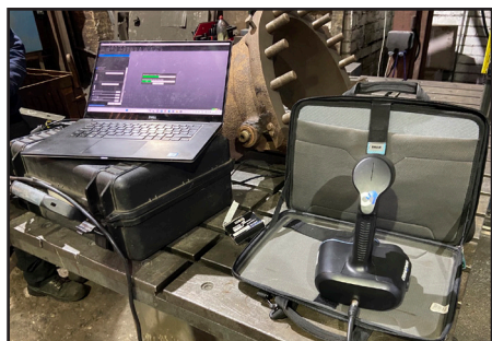
The computer and 3D scanner (all images: Boro Foundry)
