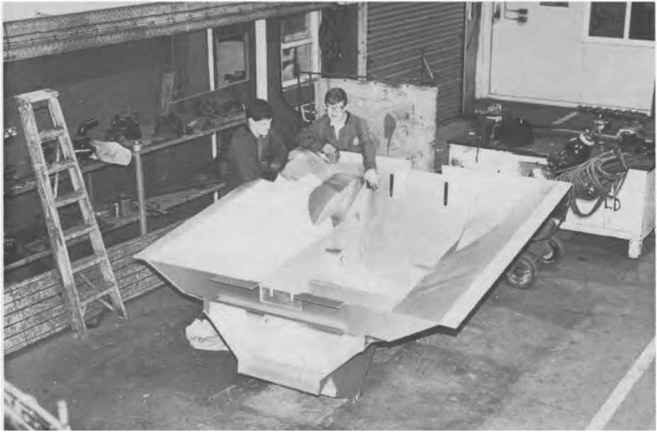
Richard and Dave Pearson take a close look at Blue Peter's new ashpan. This huge fabrication, made by the M.S.C. team, measures 50 square feet.
