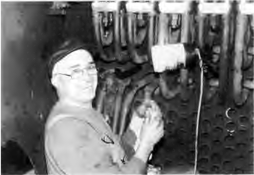
New Committee member Martin Lloyd takes a break from working on the superheater elements of the K1 at ICI Wilton on 14th May 1998 (Colin Smith)
