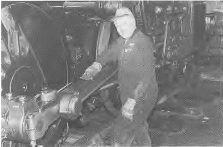
With assembly of the K1 all but complete Derek Shorten sets about cleaning the motion on 16th July (Colin Smith)
