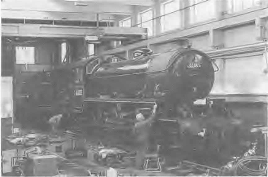
A final glimpse inside No.5 depot at Wilton on 13th August with Len Clarke touching up the lining and Eric Nott overseeing work on refitting the shortened drawbar (John Hunt)
