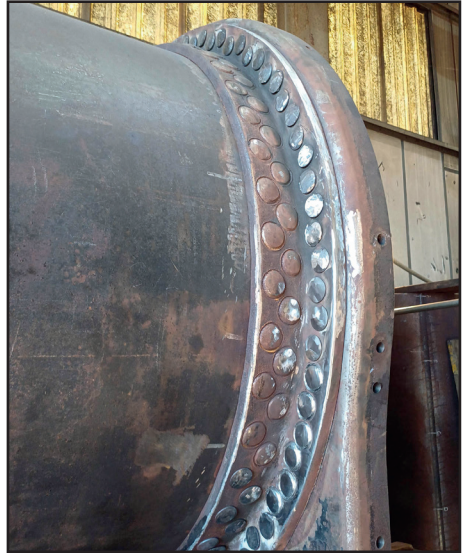
Caulking of the front tubeplate (left) and the front of the boiler barrel ring showing caulking (right) (both Dave Pennock)
