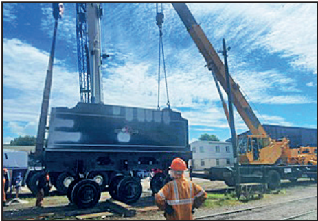
The K1 tender being renbeeled on 26th June (Lizzie Fielding) and the tender with the left-hand frames in gloss and the new running plate over the rear bufferbeam (Paul Hutchinson)
