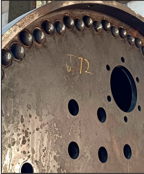
Caulking of the front tubeplate (left) and the front of the boiler barrel ring showing caulking (right) (both Dave Pennock)
