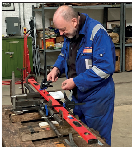
Dennis Paling taking measurements of the J72 slide valve yolk on 6th June (Colin Smith)
