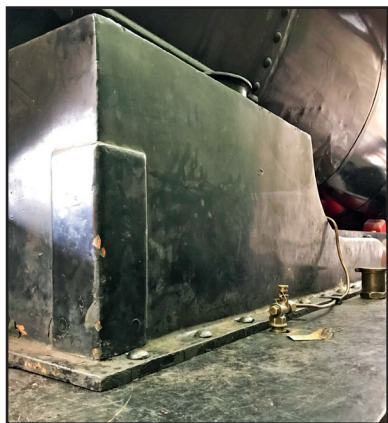
Left: the area where the new cylinder will be fitted cleaned up and painted. Right: the left-hand front sand box back in place (both Ian Pearson)
