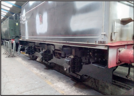
The K1 tender being renbeeled on 26th June (Lizzie Fielding) and the tender with the left-hand frames in gloss and the new running plate over the rear bufferbeam (Paul Hutchinson)
