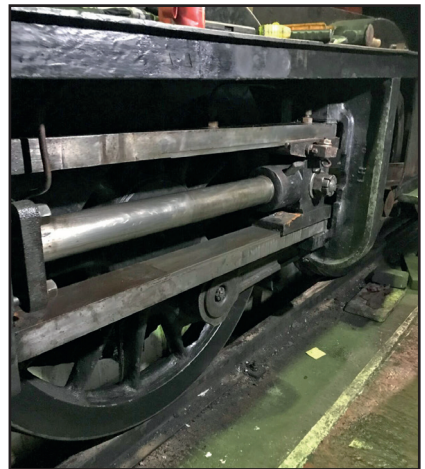
The LH piston rod and crosshead refitted on 29th October (Ian Pearson)
