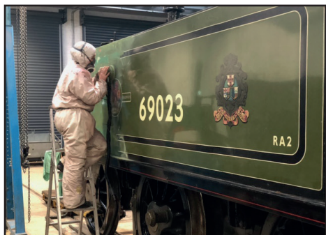
Early stages in preparing the tank sides for a new coat of paint, lining and lettering on 25th November (Ed Bolam)
