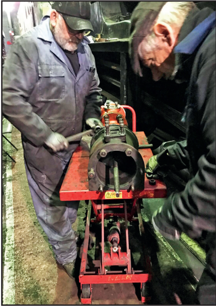
Left: Bill Dobson (right) and David Collins work on the steam reverser on 5th November (Ian Pearson) Right: The steam reverser back between the frames on 27th November, showing the restricted space in which to manoeuvre a very heavy and unwieldy piece of equipment (John Hunt)
