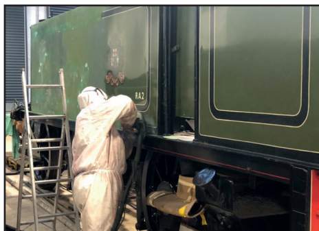
Early stages in preparing the tank sides for a new coat of paint, lining and lettering on 25th November (Ed Bolam)
