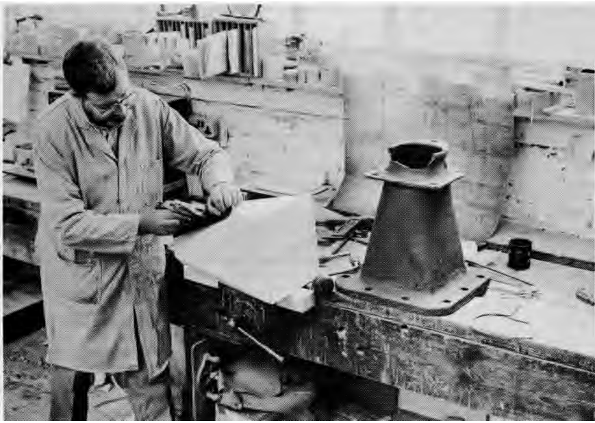
A pattern maker at Stockton Castings Ltd works on the new pattern for the K1's blastpipe, using an L.N.E.R. drawing and the original blastpipe as guidance, on 20th September, 24 hours after the defect was found. (Maurice Burns)
