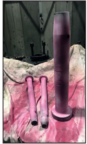
Various drawbar pins and linkages after dye penetration testing on 28th January (Ian Pearson)
