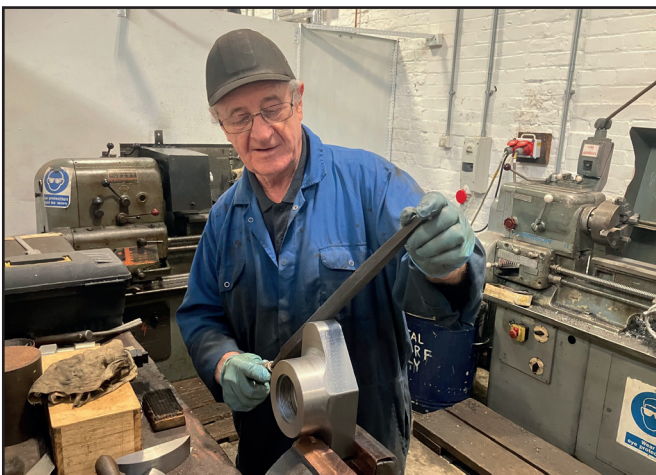
Arthur Jenkins works on the cylinder relief adapters for the Q6 cylinder relief valves (Neal Woods)
