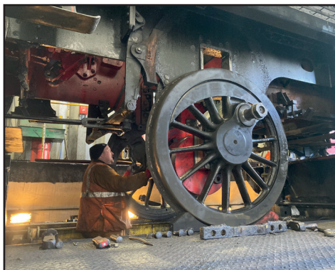
The P3's centre wheelset being lowered out on the wheel drop on 8th January (Richard Pearson)
