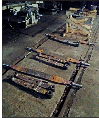
Left: the tender front on 23rd December (Paul Hutchinson) Right: tender brake tables with their refurbished journals and rebushed hangers (Paul Hutchinson)
