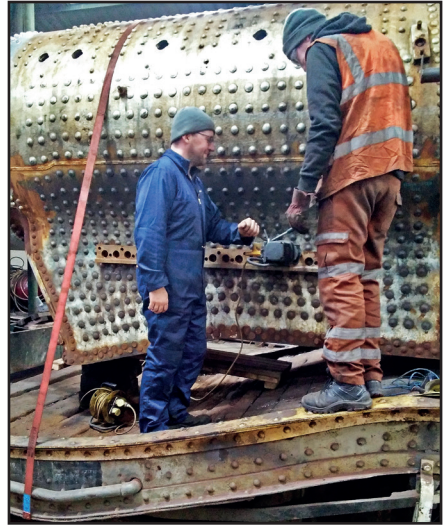
Chris Williams and Kenny Morrison drilling expansion bracket stud holes (Paul Hutchinson)
