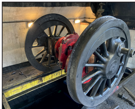
The P3's centre wheelset being lowered out on the wheel drop on 8th January (Richard Pearson)
