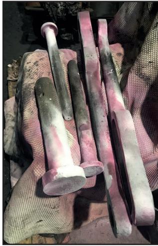
Various drawbar pins and linkages after dye penetration testing on 28th January (Ian Pearson)
