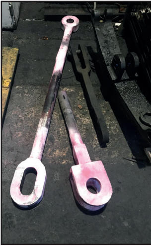
Various drawbar pins and linkages after dye penetration testing on 28th January (Ian Pearson)
