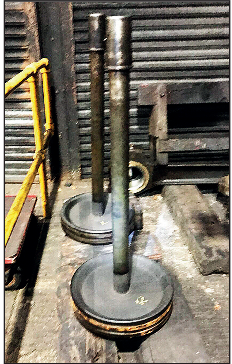
Left: The front end of the P3 with the valves and pistons removed on 2nd January; this involved removing the buffer beam (Ian Pearson). Right: The two pistons awaiting attention on the same day (Ian Pearson)
