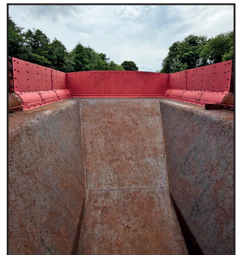
Following rewheeling some paintwork was touched up and the coal space was cleaned ready for protective painting (Ian Pearson)
