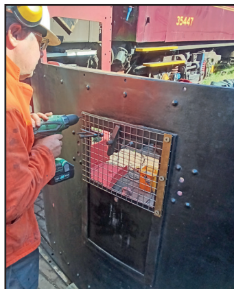
Below: Wayne Denney fitting the new cab roof vent safety mesh (all Paul Hutchinson)
