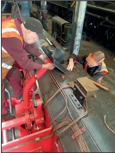
Left: Steve Gibson and Les Harper fitting the LH intermediate forwards sands filler pipe.
