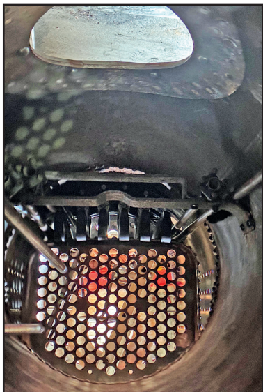
Left: the view towards the firebox tubeplate, showing the girder stays, with the dome hole at the top, and the longitudinal stays fitted to date and internal water feed/ steam pipework.
