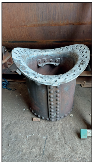
Right: the cracking in the flange that requires welding (Neal Woods)
