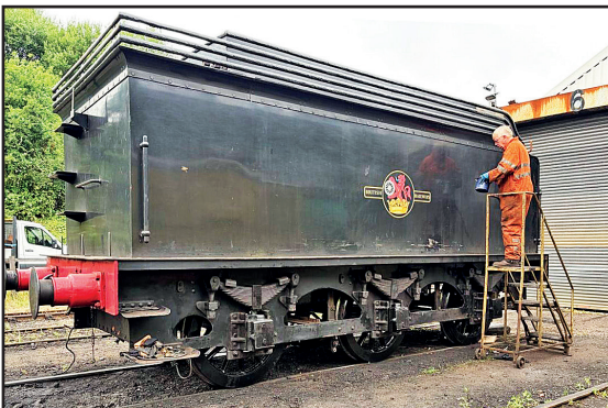
Following rewheeling some paintwork was touched up and the coal space was cleaned ready for protective painting (Ian Pearson)
